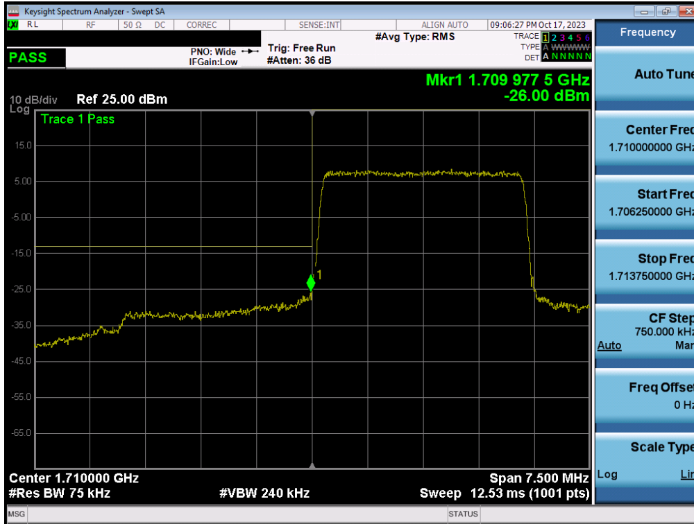
Plot 7-103. Lower Band Edge Plot (LTE Band 66/4 - 3MHz QPSK – Full RB - Ant1)
