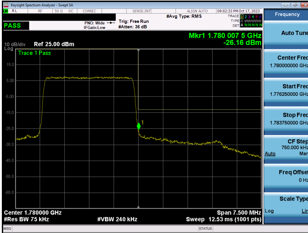
Plot 7-107. Upper Band Edge Plot (LTE Band 66 - 3MHz QPSK – Full RB - Ant1)
