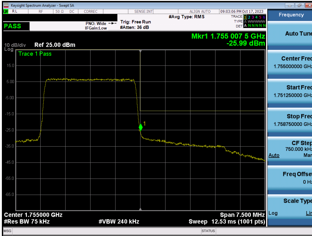
Plot 7-105. Upper Band Edge Plot (LTE Band 4 - 3MHz QPSK – Full RB - Ant1)
