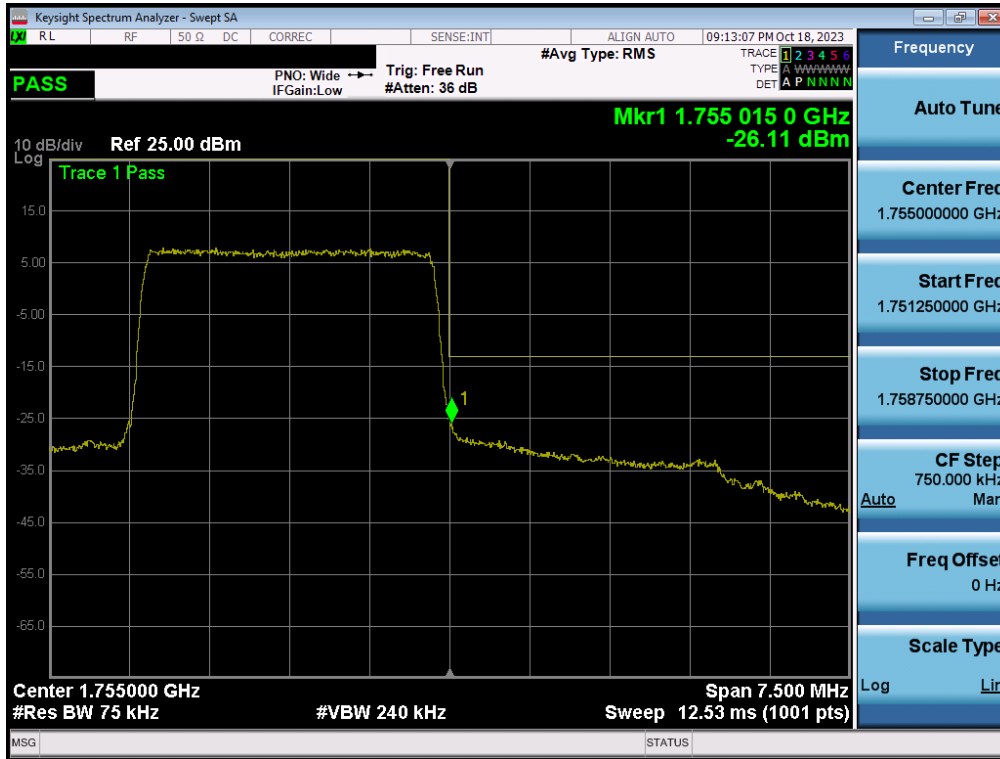
Plot 7-111. Upper Band Edge Plot (LTE Band 4 - 3MHz QPSK – Full RB - Ant2)
