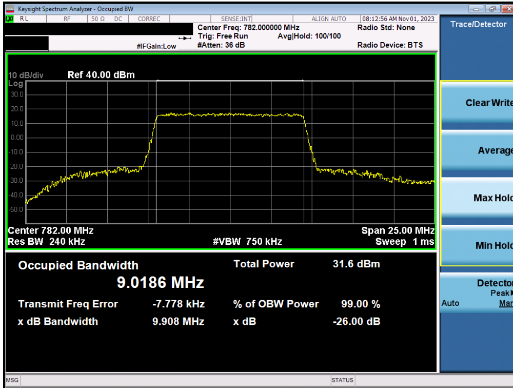
Plot 7-9. Occupied Bandwidth Plot (LTE Band 13 - 10MHz QPSK - Full RB – Ant1)
