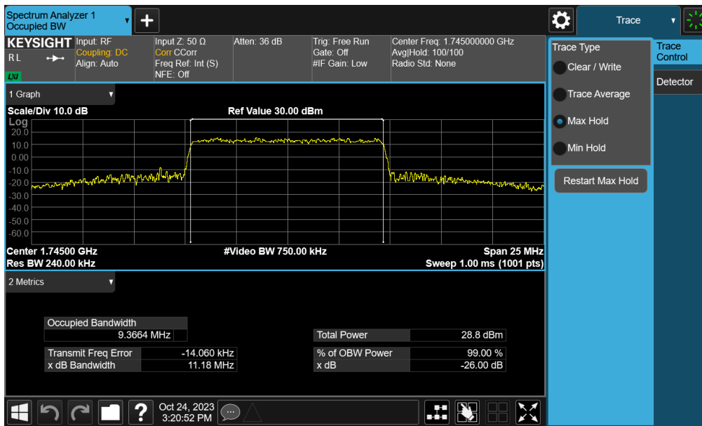
Plot 7-69. Occupied Bandwidth Plot (NR Band n66 - 10.0MHz QPSK - Full RB - Ant2)
