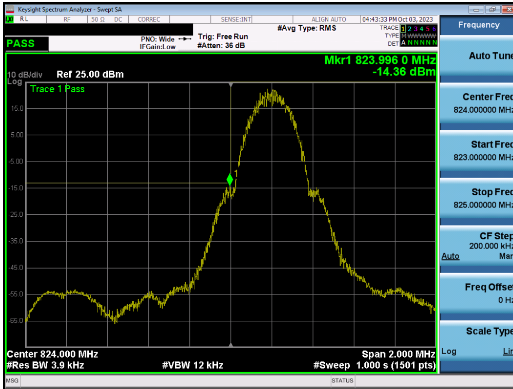
Plot 7-42. Lower Band Edge Plot (GPRS Cell – Ch. 128)
