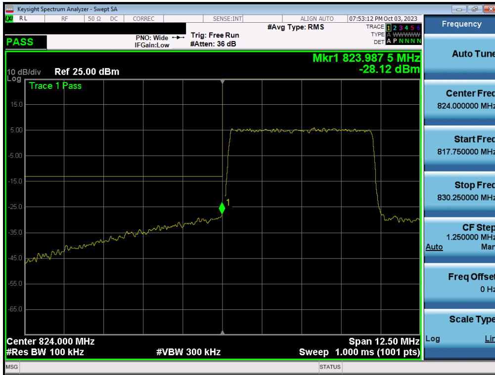
Plot 7-40. Lower Band Edge Plot (NR Band n5 – 5.0MHz - Full RB)
