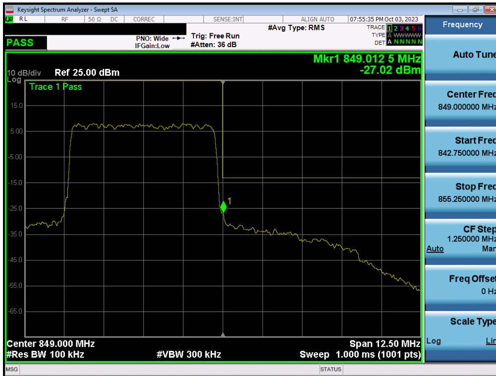
Plot 7-41. Upper Band Edge Plot (NR Band n5 – 5.0MHz - Full RB)
