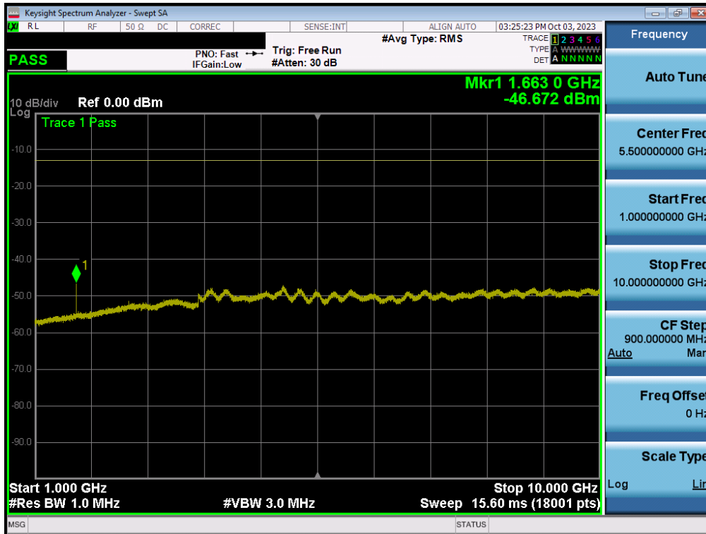
Plot 7-28. Conducted Spurious Plot (LTE Band 26/5 - 10MHz QPSK - 1 RB - Low Channel)
