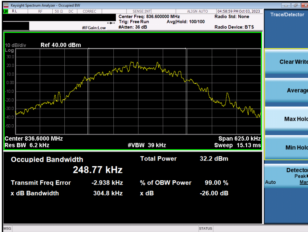
Plot 7-24. Occupied Bandwidth Plot (EDGE, Ch. 190)
