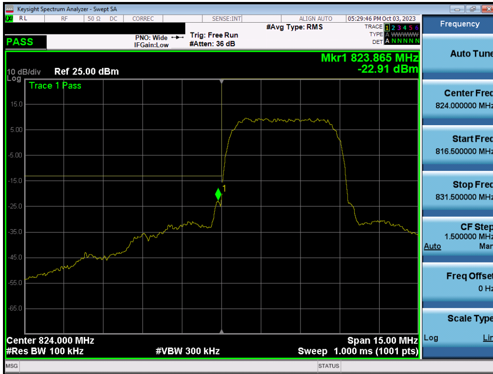
Plot 7-44. Lower Band Edge Plot (WCDMA Cell – Ch. 4132)
