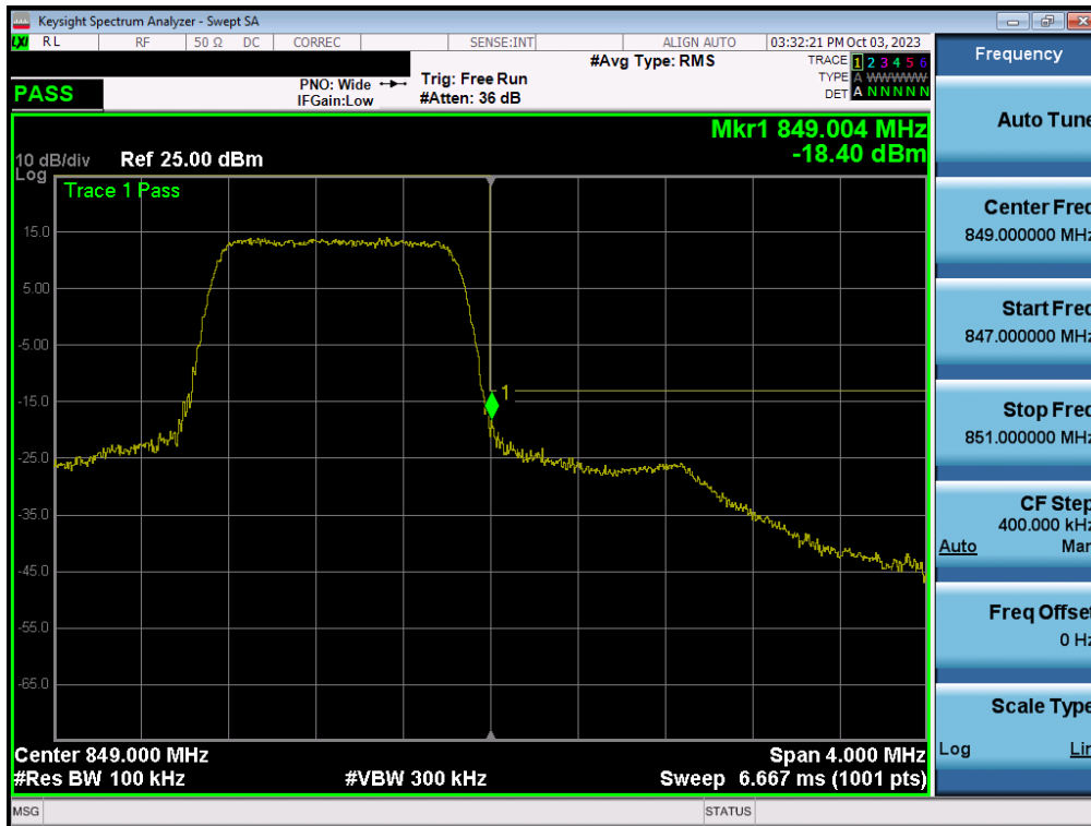
Plot 7-39. Upper Band Edge Plot (LTE Band 26/5 – 1.4MHz QPSK – Full RB)
