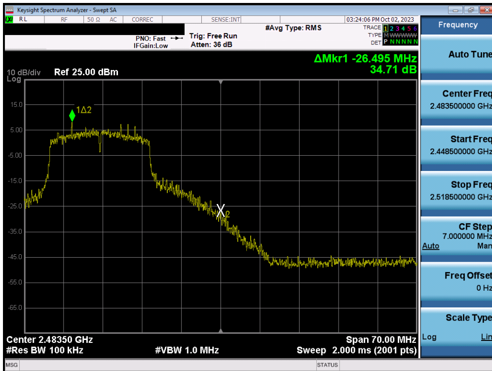
Plot 7-28. Band Edge Plot (802.11n (2.4GHz) – Ch. 11)
