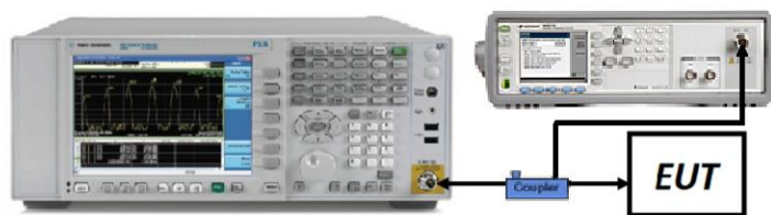
Figure 7-4. Test Instrument & Measurement Setup
