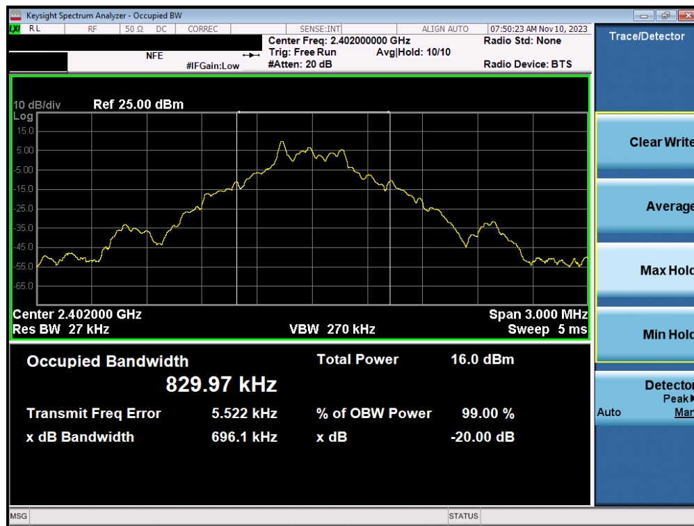
Plot 7-1. 20dB Bandwidth Plot (Bluetooth, 1Mbps – Ch. 0)
