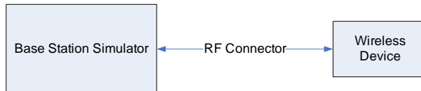
Figure 10-3 Power Measurement Setup
