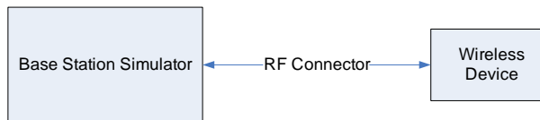
Figure 10-4 Power Measurement Setup – NR FDD
