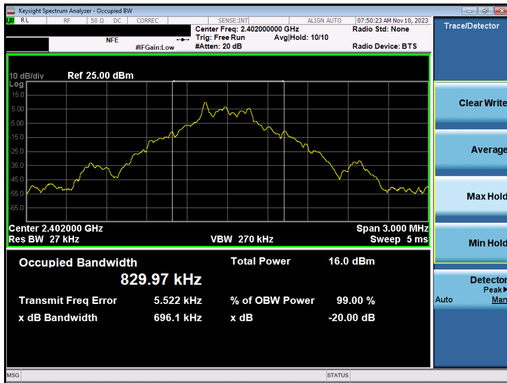
Plot 7-1. 20dB Bandwidth Plot (Bluetooth, 1Mbps – Ch. 0)
