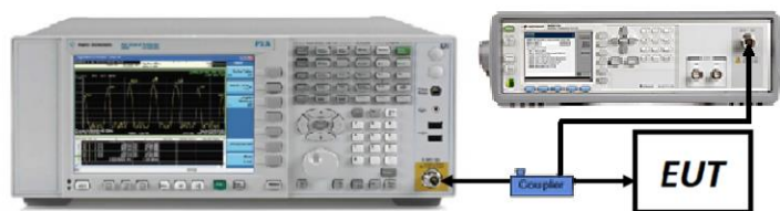
Figure 7-2. Test Instrument & Measurement Setup
