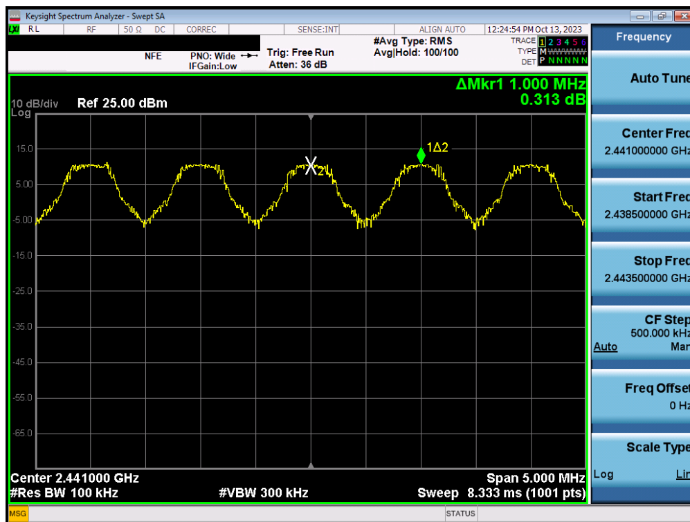
Plot 7-32. Channel Spacing Plot (Bluetooth)
