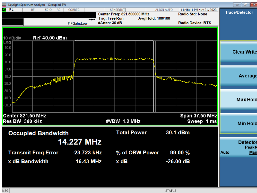
Plot 7-16. Occupied Bandwidth Plot (NR Band n26 - 15MHz 16-QAM - Full RB Configuration)
