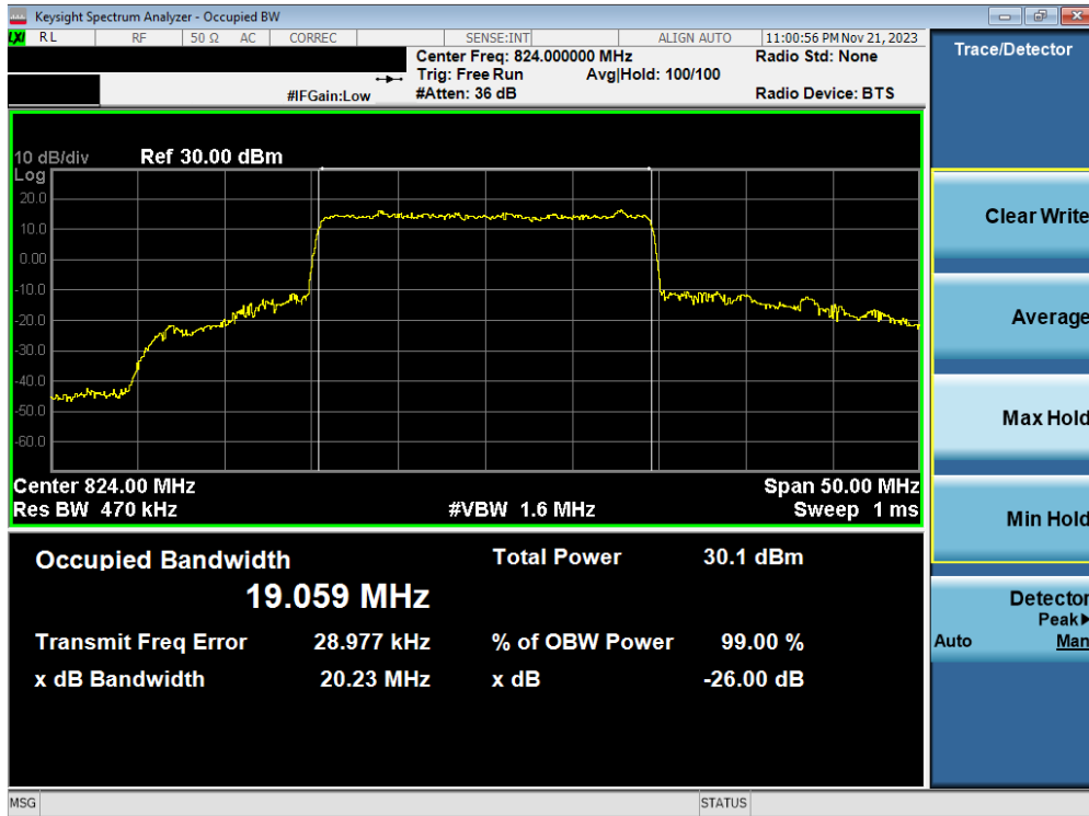
Plot 7-12. Occupied Bandwidth Plot (NR Band n26 - 20MHz QPSK - Full RB Configuration)
