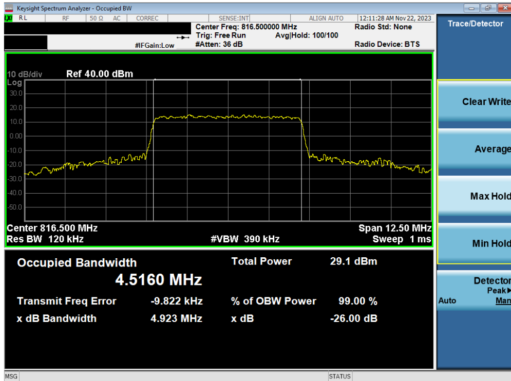
Plot 7-22. Occupied Bandwidth Plot (NR Band n26 - 5MHz 16-QAM - Full RB Configuration)
