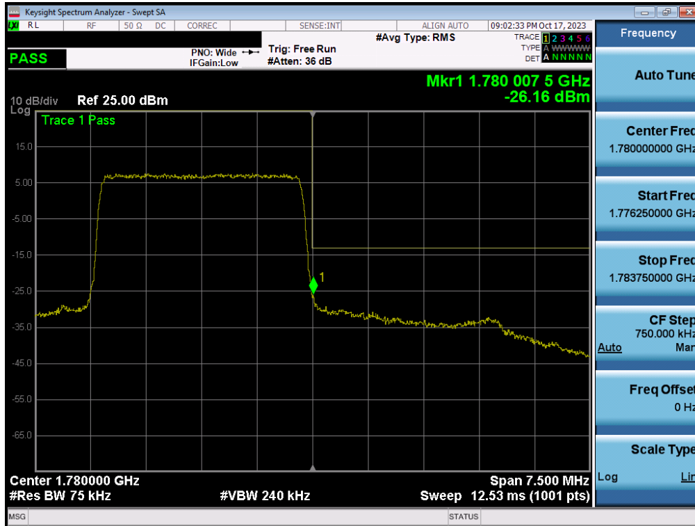
Plot 7-98. Upper Band Edge Plot (LTE Band 66 - 3MHz QPSK – Full RB - Ant1)
