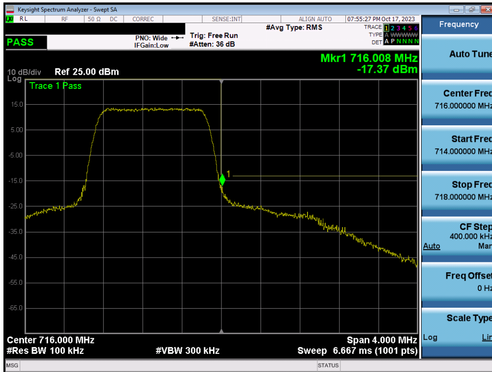
Plot 7-89. Upper Band Edge Plot (LTE Band 12 – 1.4MHz QPSK – Full RB - Ant1)
