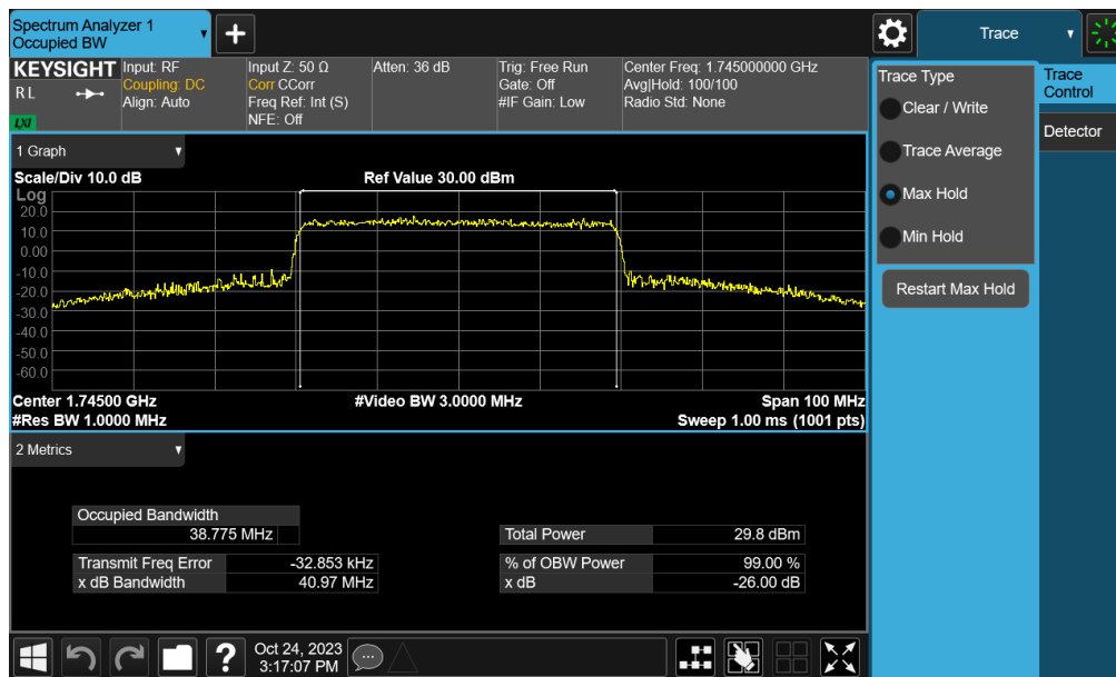
Plot 7-54. Occupied Bandwidth Plot (NR Band n66 - 40.0MHz 16QAM - Full RB – Ant2)
