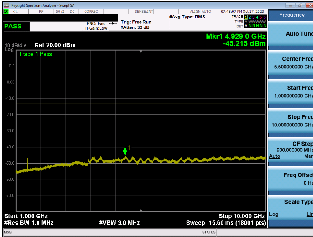
Plot 7-72. Conducted Spurious Plot (LTE Band 12/17 - 10MHz QPSK - 1 RB - High Channel - Ant1)
