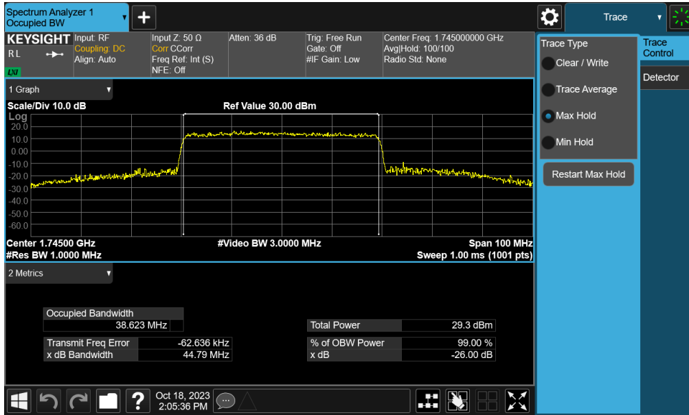
Plot 7-35. Occupied Bandwidth Plot (NR Band n66 - 40.0MHz QPSK - Full RB – Ant1)
