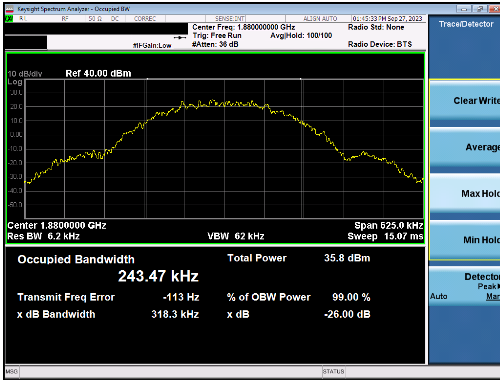
Plot 7-25. Occupied Bandwidth Plot (GPRS, Ch. 661 - Ant1)
