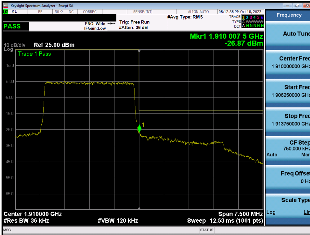
Plot 7-46. Upper Band Edge Plot (LTE Band 2 - 3MHz QPSK – Full RB - Ant2)
