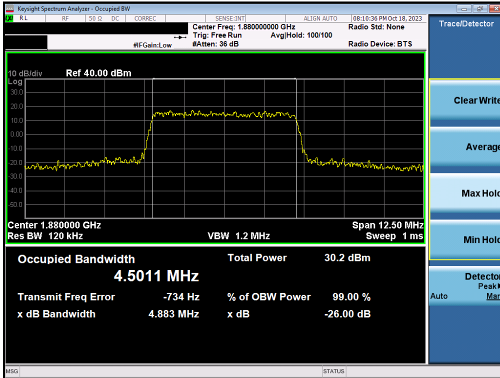
Plot 7-19. Occupied Bandwidth Plot (LTE Band 2 - 5MHz QPSK - Full RB - Ant2)
