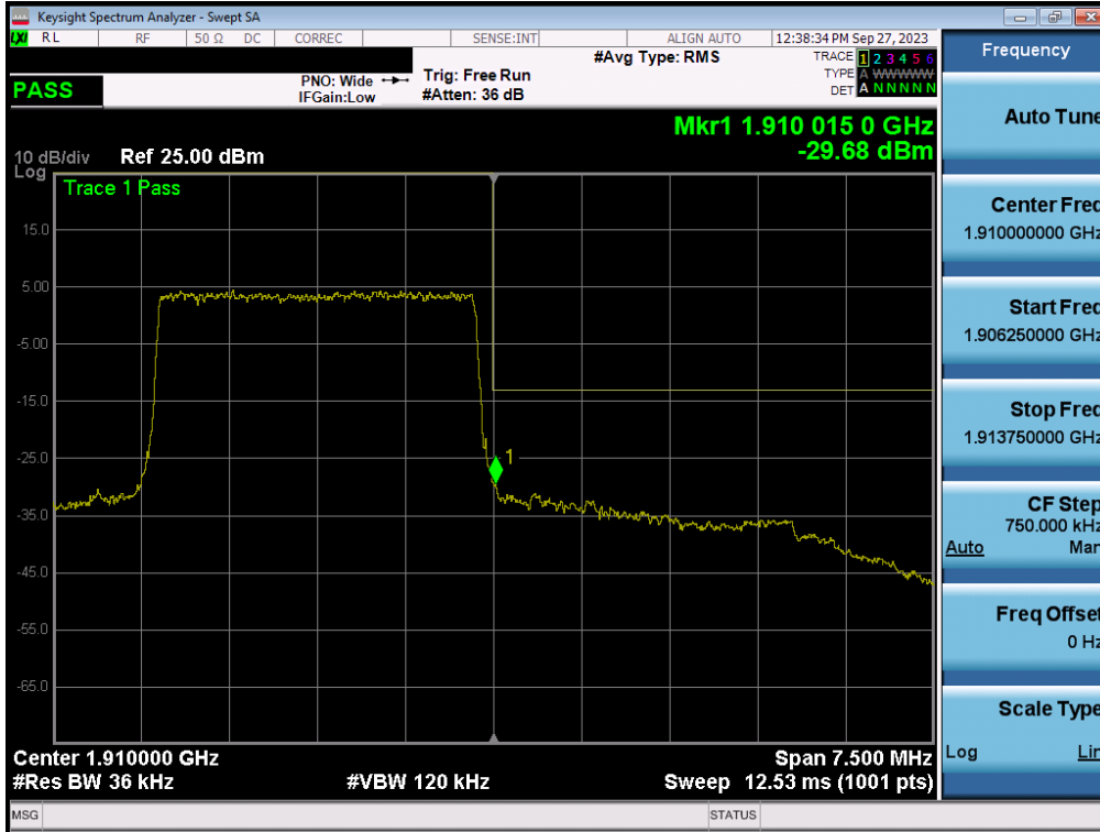
Plot 7-42. Upper Band Edge Plot (LTE Band 2 - 3MHz QPSK – Full RB - Ant1)
