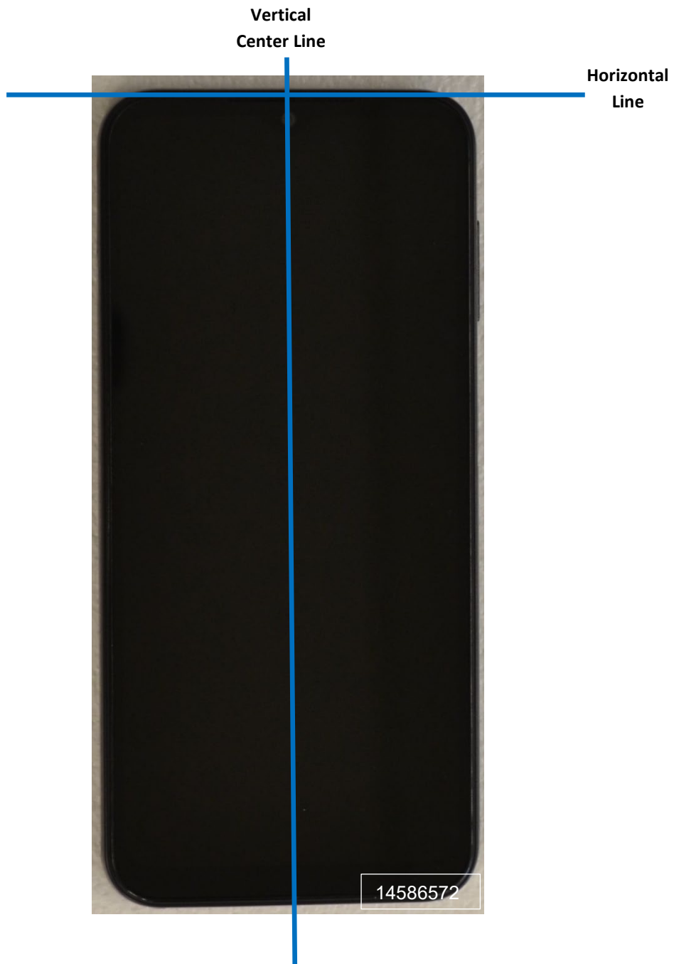
Photograph 4: Handset Vertical and Horizontal Reference Lines
