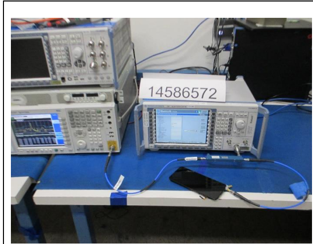
RF ANTENNA PORT CONDUCTED
