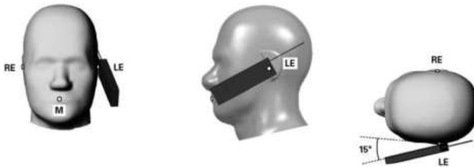
Figure 8.5. Tilt 15° position of the wireless device
