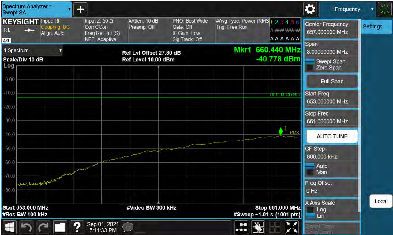
Sub6 n71. Lower Extended Band Edge Plot (20 M BW Ch.134600 BPSK_ Full RB)
