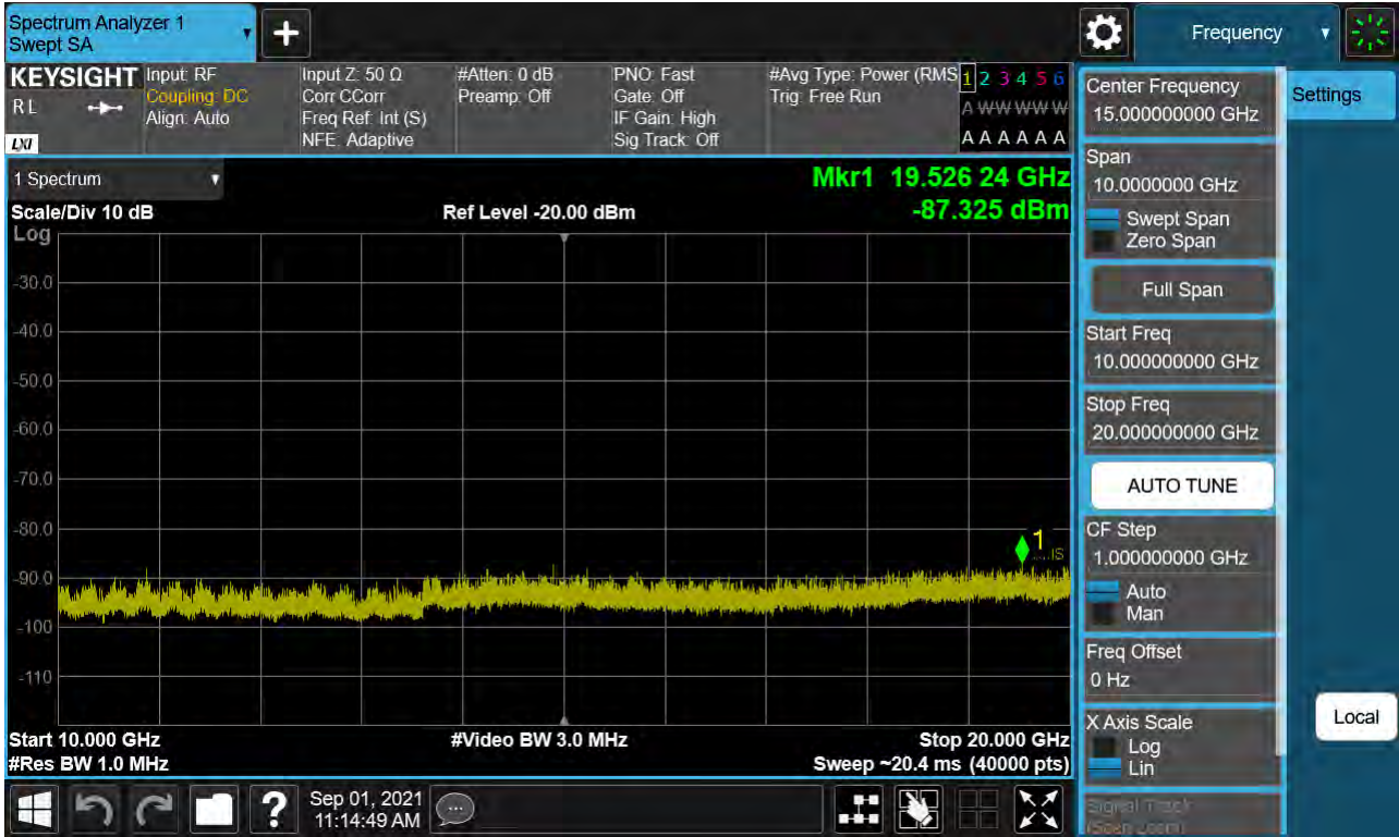
Sub6 n66. Conducted Spurious Plot_2 (355000ch_10 MHz_BPSK_RB 1_1)
