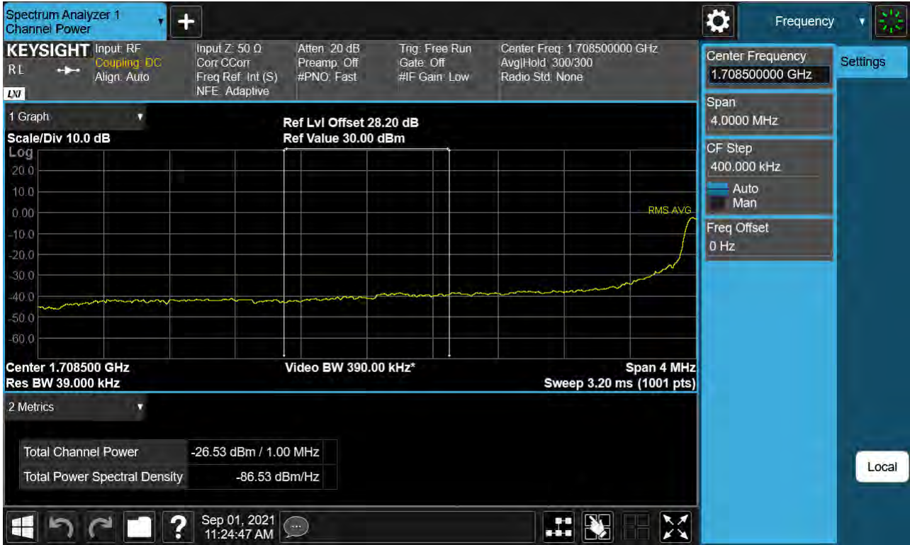
Sub6 n66. Lower Extended Band Edge Plot (20 M BW Ch.344000 BPSK_ Full RB) -3
