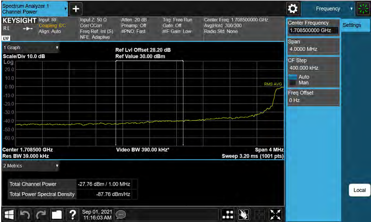
Sub6 n66. Lower Extended Band Edge Plot (15 M BW Ch.343500 BPSK_ Full RB) -3
