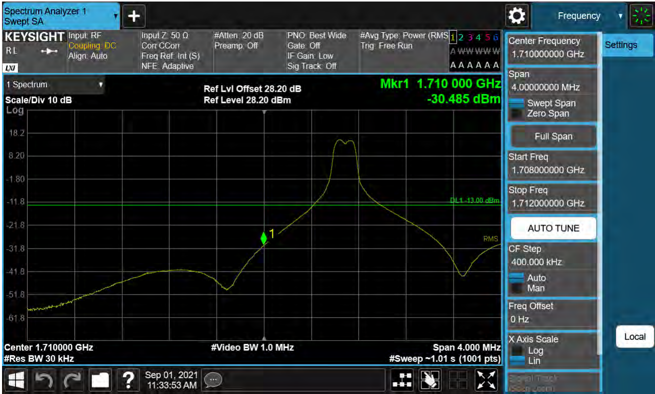
Sub6 n66. Lower Band Edge Plot (30 M BW Ch.345000 BPSK RB 1, Offset 0) -1
