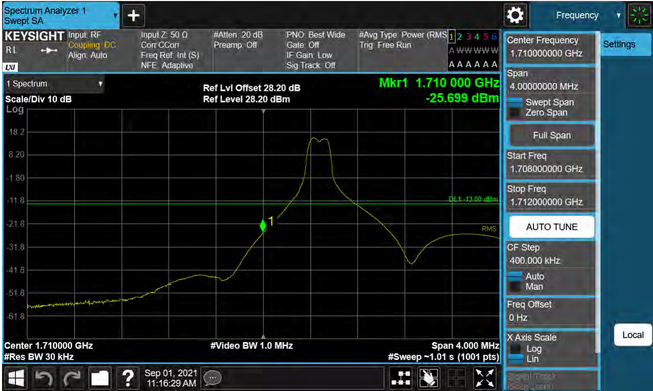
Sub6 n66. Lower Band Edge Plot (15 M BW Ch.343500 BPSK RB 1, Offset 0) -1
