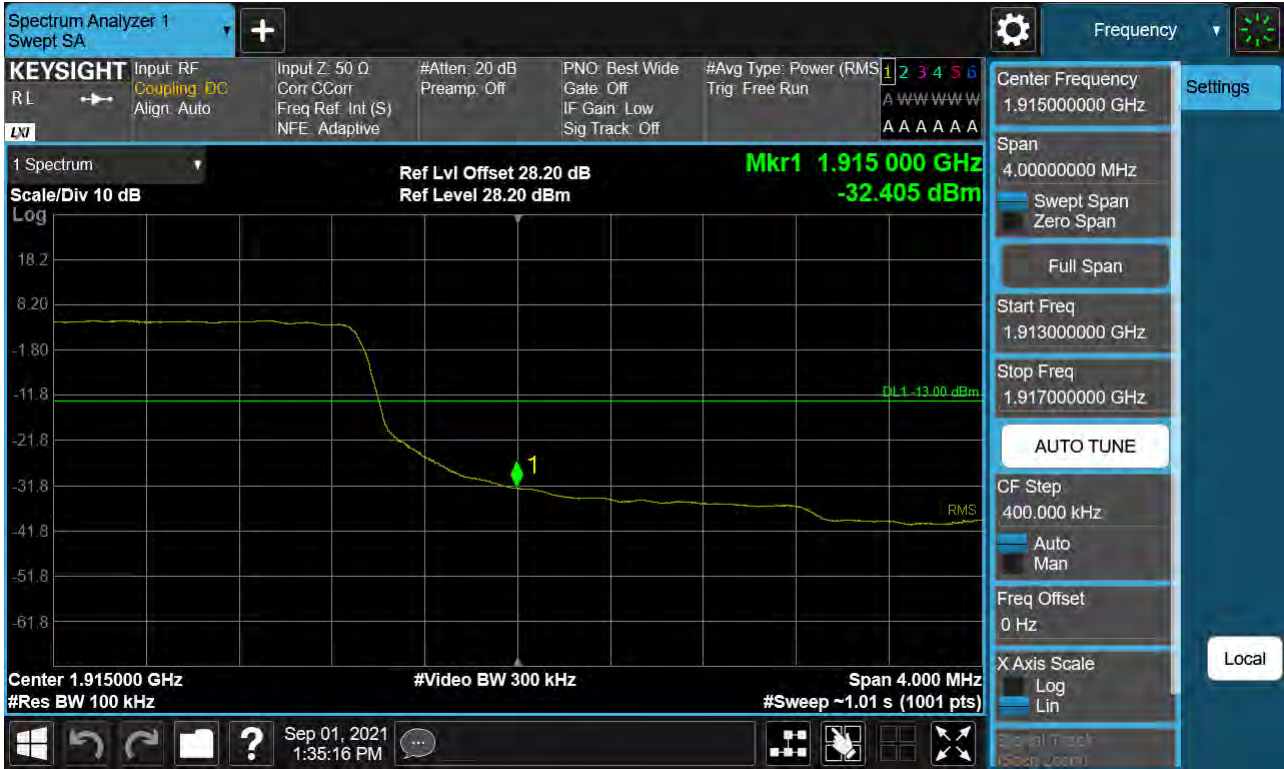
Sub6 n25(2). Upper Band Edge Plot (10 M BW Ch.382000 BPSK_ Full RB) -1
