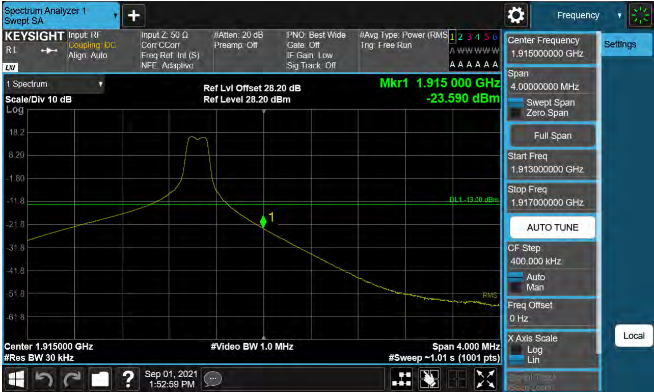
Sub6 n25(2). Upper Band Edge Plot (20 M BW Ch.381000 BPSK_RB1_Offset 105)
