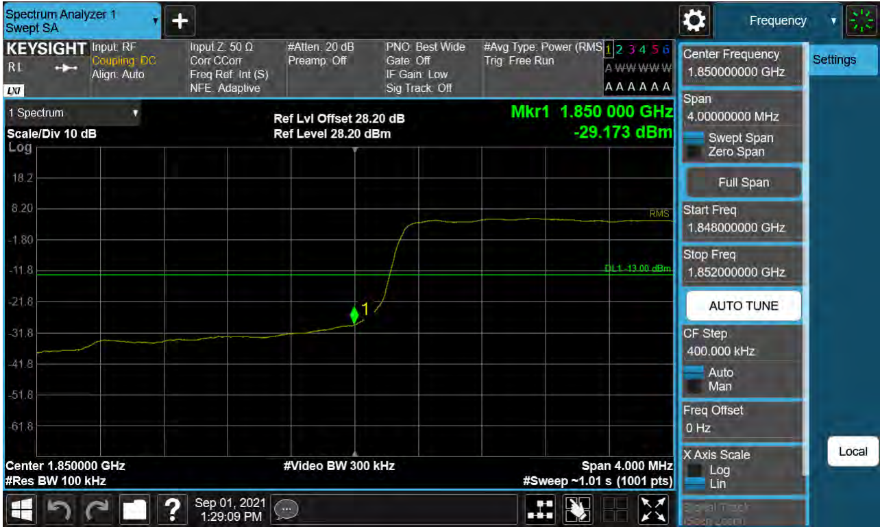
Sub6 n25(2). Lower Band Edge Plot (10 M BW Ch.371000 BPSK_ Full RB) -1
