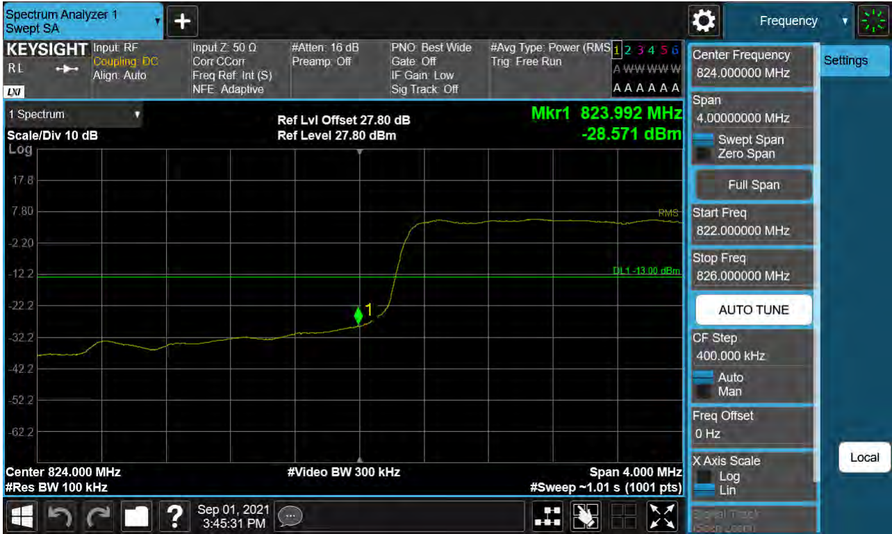
Sub6 n5. Lower Band Edge Plot (10 M BW Ch.165800 BPSK_ Full RB)
