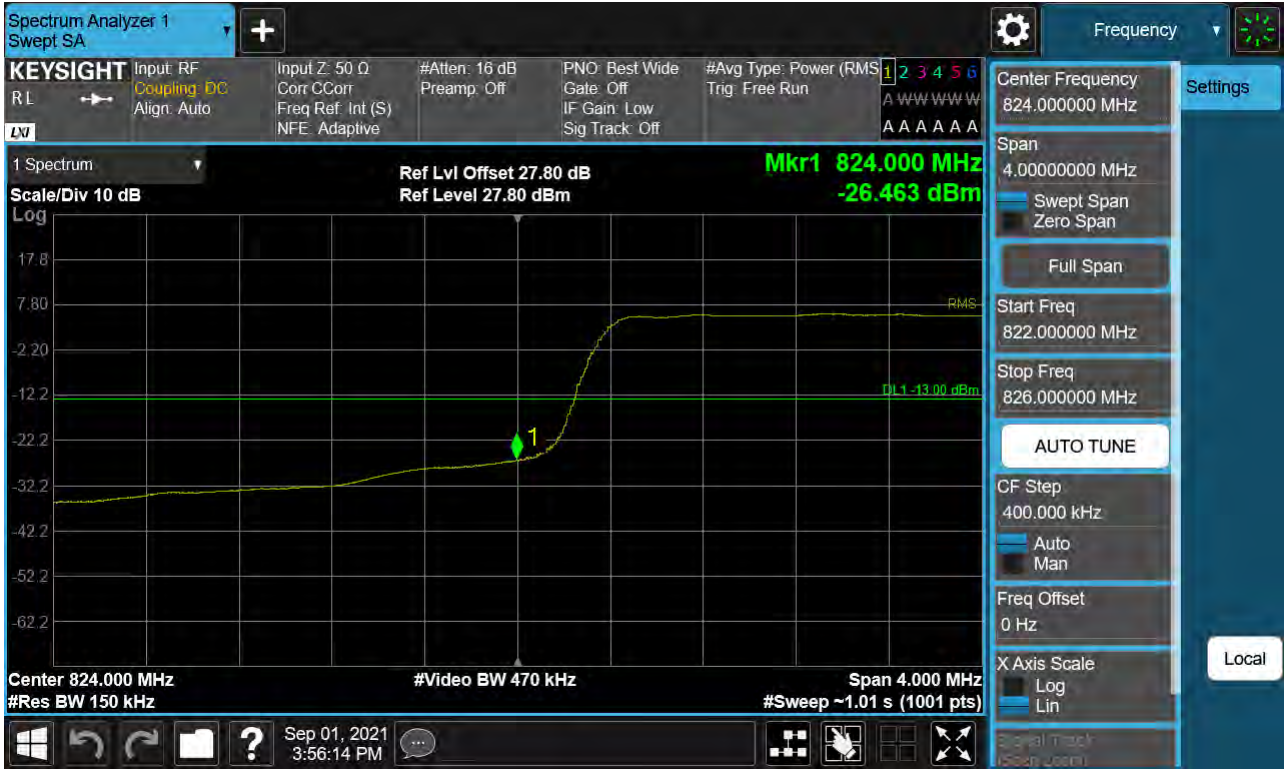
Sub6 n5. Lower Band Edge Plot (15 M BW Ch.166300 BPSK_ Full RB)
