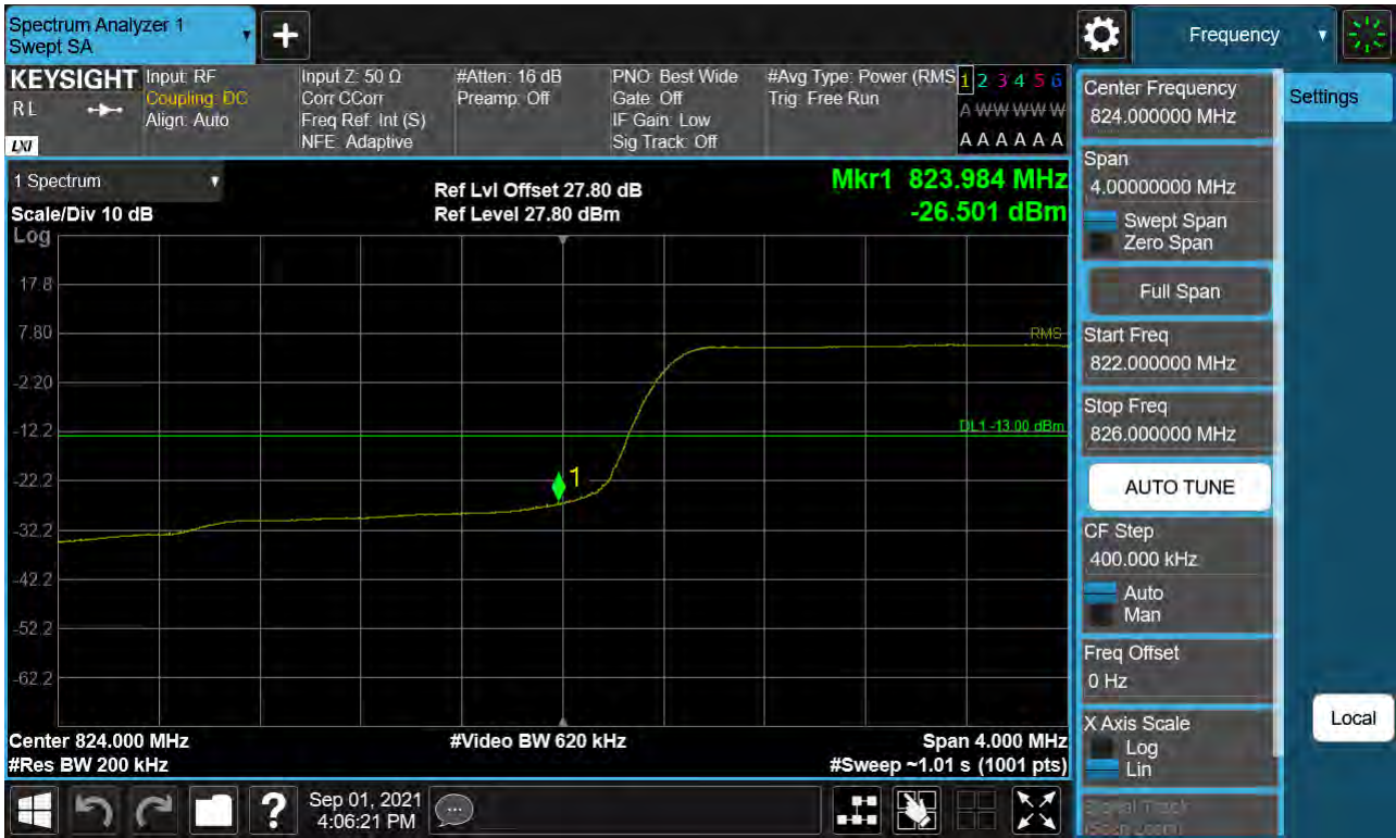
Sub6 n5. Lower Band Edge Plot (20 M BW Ch.166800 BPSK_ Full RB)
