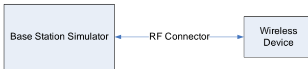
Figure 9-1 Power Measurement Setup
