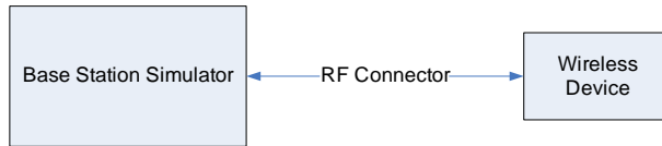
Figure 9-3 Power Measurement Setup
