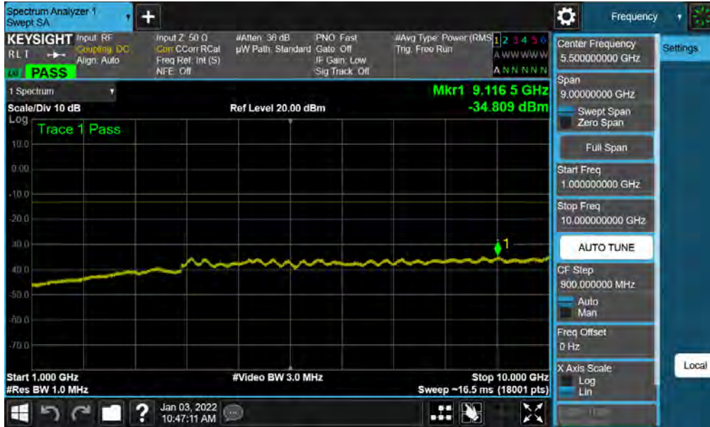
Plot 7-20. Conducted Spurious Plot (LTE Band 26 - 15MHz QPSK - RB Size 1, RB Offset 0)
