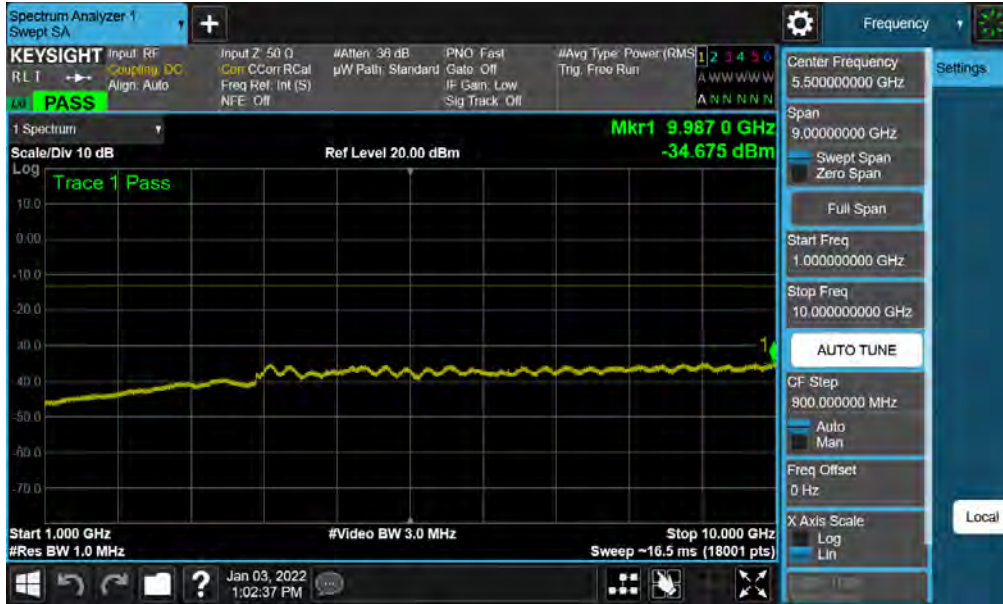
Plot 7-17. Conducted Spurious Plot (LTE Band 14 - 10MHz QPSK - RB Size 1, RB Offset 0)
