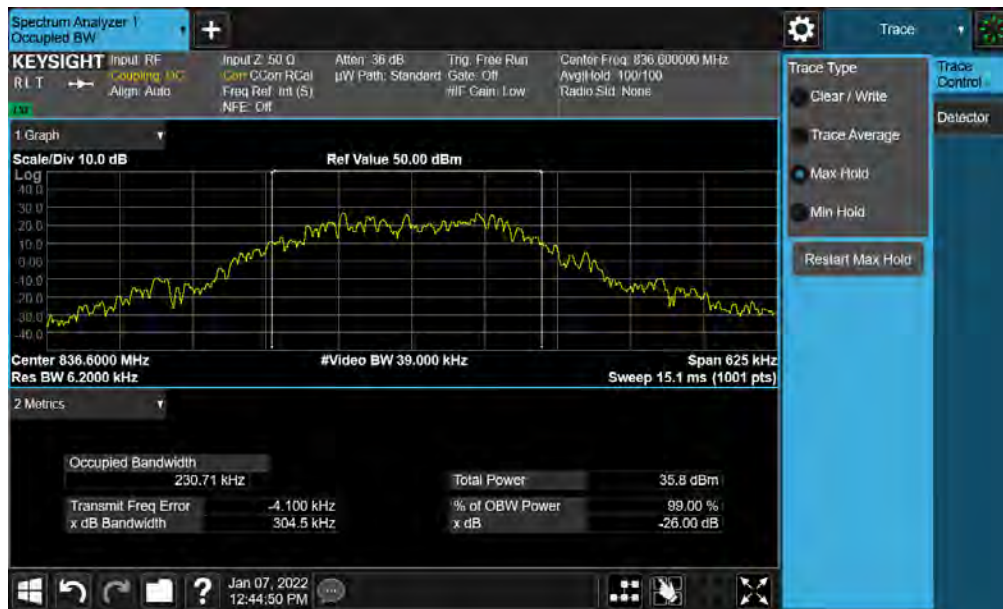
Plot 7-12. Occupied Bandwidth Plot (EDGE, Ch. 190)
