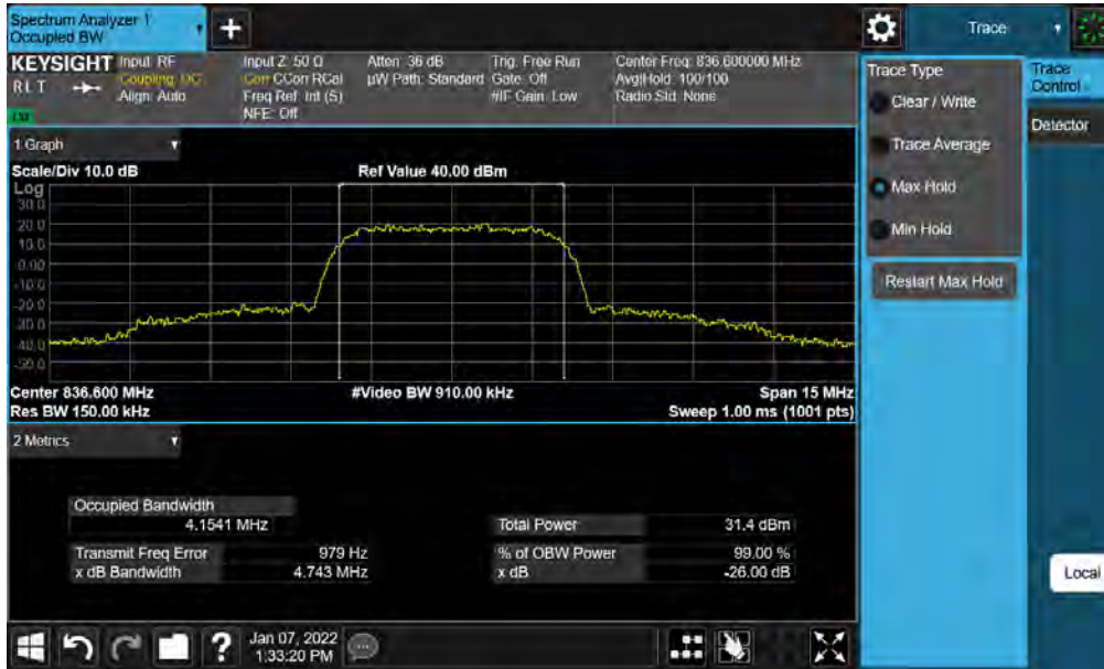
Plot 7-13. Occupied Bandwidth Plot (WCDMA, Ch. 4183)
