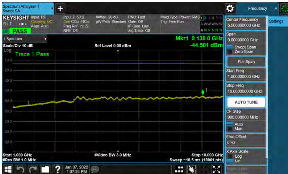
Plot 7-37. Conducted Spurious Plot (WCDMA Ch. 4183)
