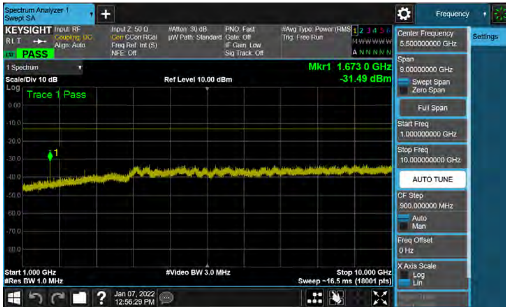
Plot 7-28. Conducted Spurious Plot (GPRS Ch. 190)
