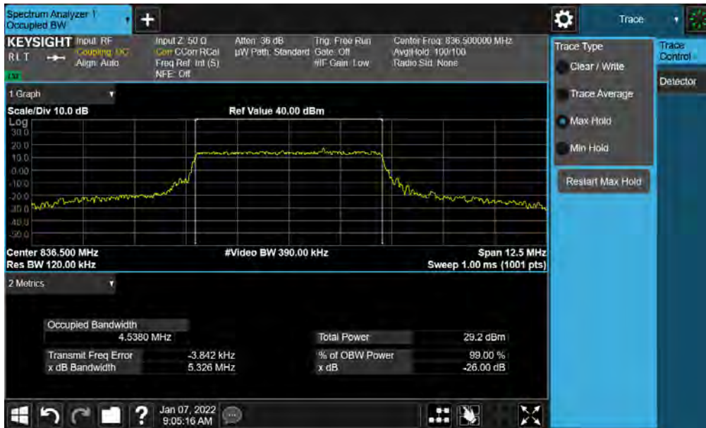
Plot 7-6. Occupied Bandwidth Plot (LTE Band 26/5 - 5MHz 16-QAM - Full RB)
