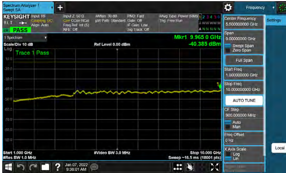
Plot 7-22. Conducted Spurious Plot (LTE Band 26/5 - 10MHz QPSK - 1 RB - High Channel)
