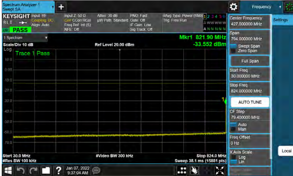
Plot 7-20. Conducted Spurious Plot (LTE Band 26/5 - 10MHz QPSK - 1 RB - High Channel)
