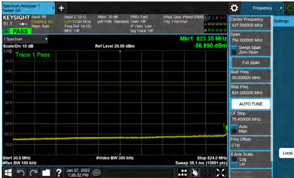
Plot 7-35. Conducted Spurious Plot (WCDMA Ch. 4183)
