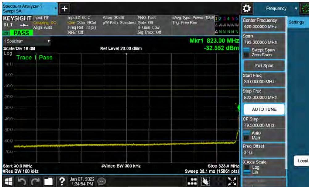
Plot 7-32. Conducted Spurious Plot (WCDMA Ch. 4132)
