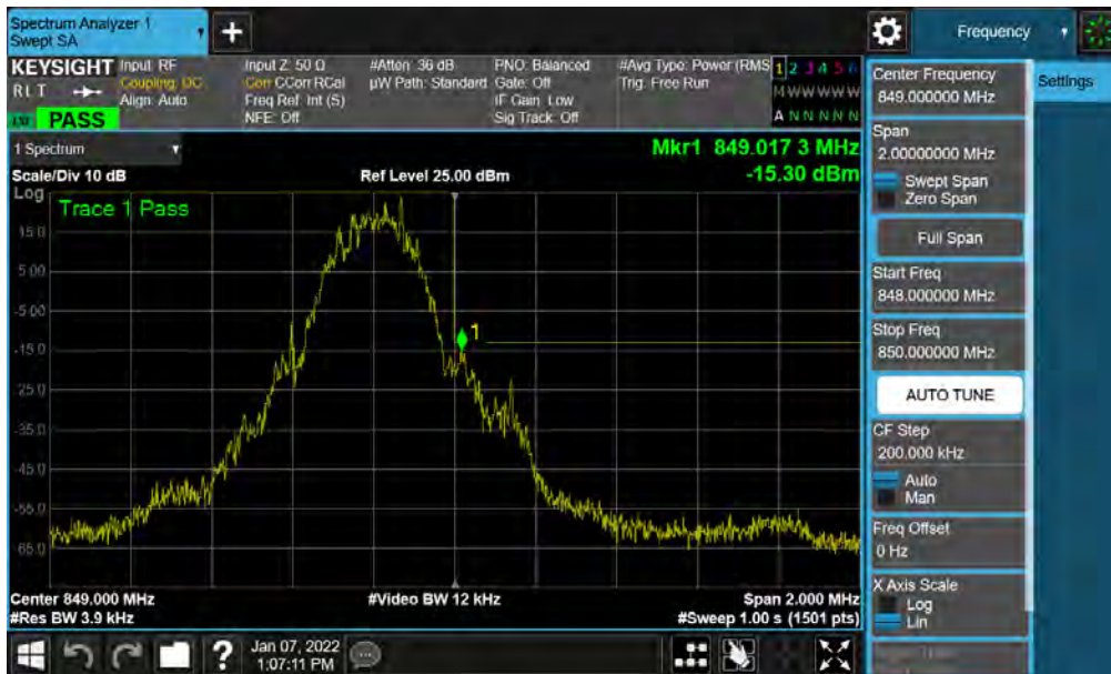
Plot 7-52. Upper Band Edge Plot (GPRS Cell – Ch. 251)
