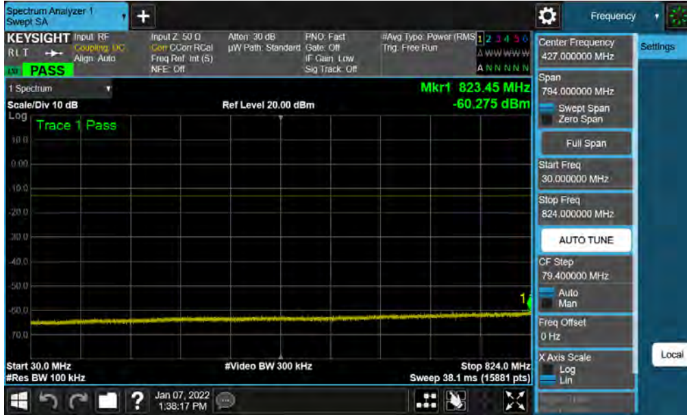
Plot 7-38. Conducted Spurious Plot (WCDMA Ch. 4233)
