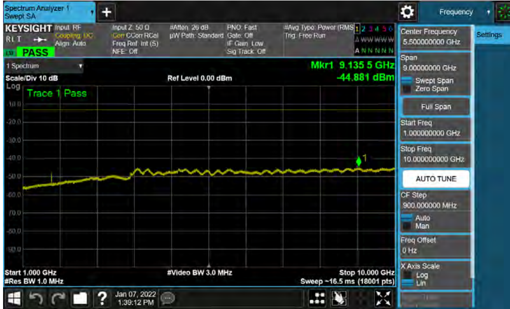
Plot 7-40. Conducted Spurious Plot (WCDMA Ch. 4233)
