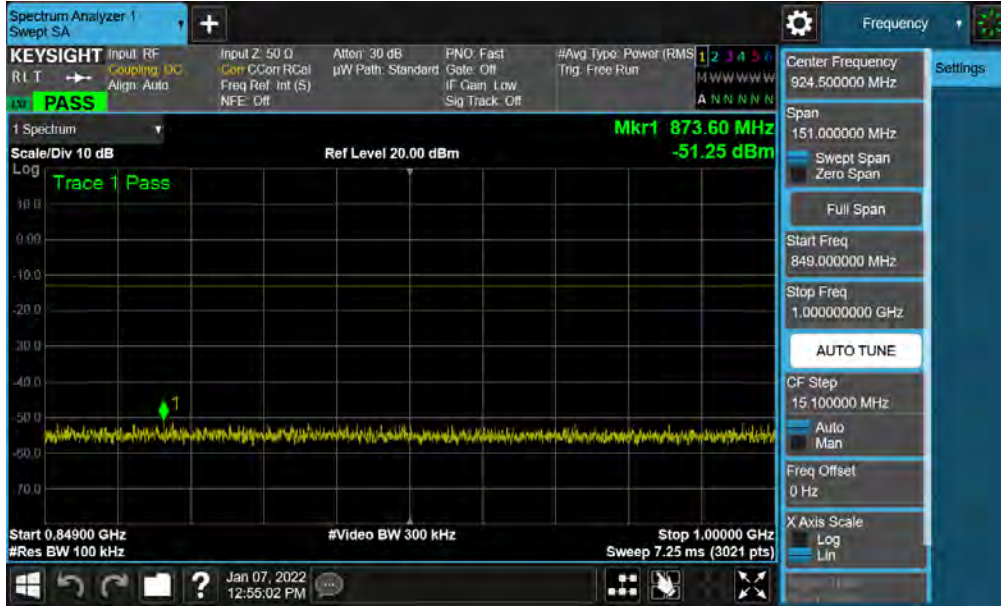
Plot 7-27. Conducted Spurious Plot (GPRS Ch. 190)
