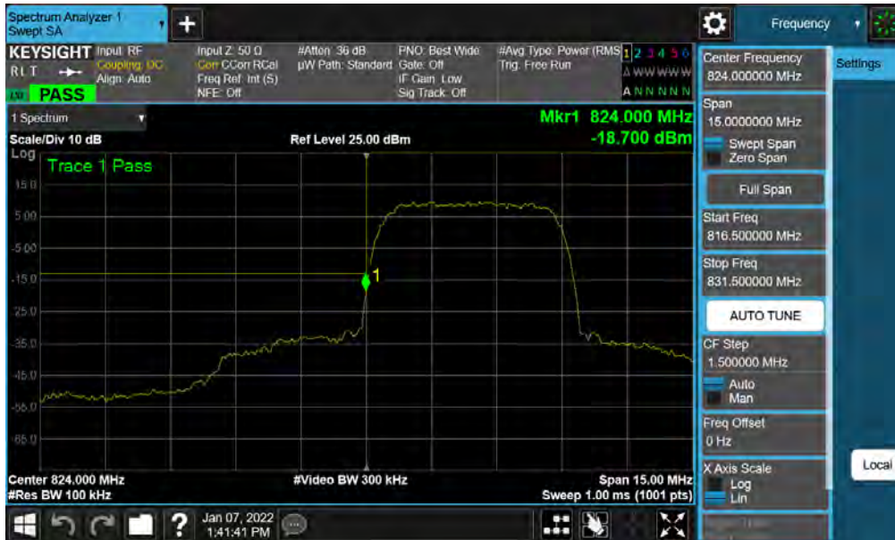
Plot 7-53. Lower Band Edge Plot (WCDMA Cell – Ch. 4132)
