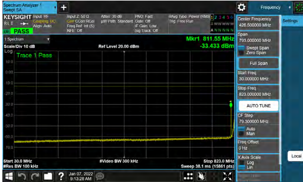
Plot 7-14. Conducted Spurious Plot (LTE Band 26/5 - 10MHz QPSK - 1 RB - Low Channel)
