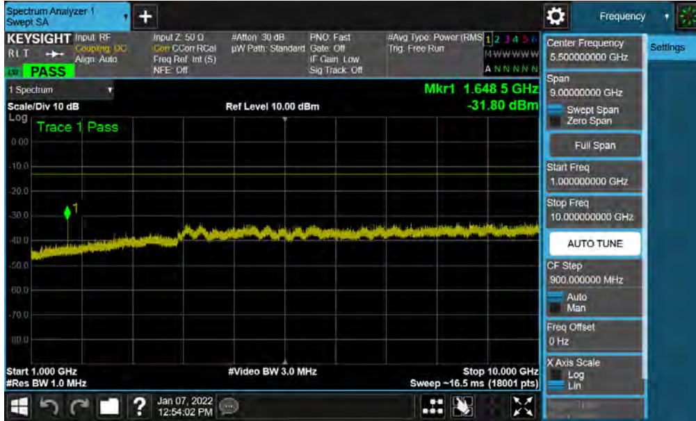
Plot 7-25. Conducted Spurious Plot (GPRS Ch. 128)
