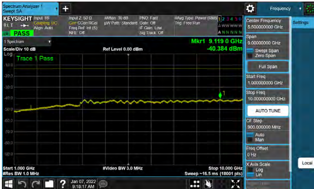
Plot 7-19. Conducted Spurious Plot (LTE Band 26/5 - 10MHz QPSK - 1 RB - Mid Channel)
