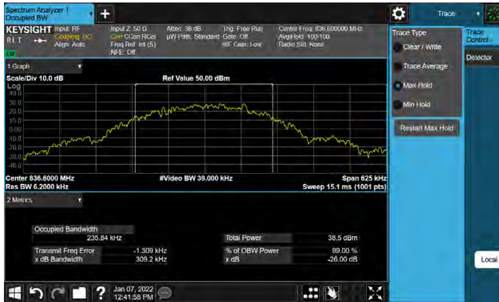
Plot 7-11. Occupied Bandwidth Plot (GPRS, Ch. 190)
