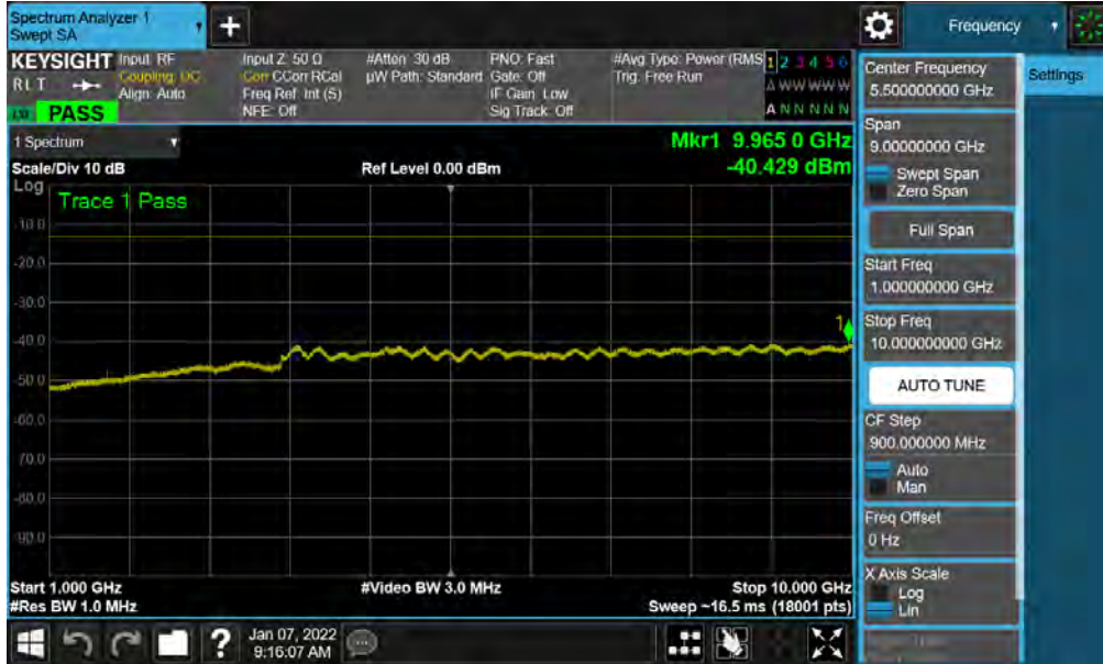
Plot 7-16. Conducted Spurious Plot (LTE Band 26/5 - 10MHz QPSK - 1 RB - Low Channel)
