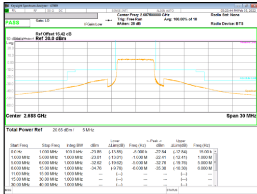
16QAM High channel FRB
