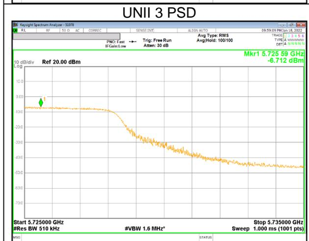
**UNII Straddle Ch. IEEE 802.11ac VHT80 mode Output Power and PSD**
