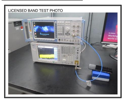
2) CONDUCTED RF MEASUREMENT SETUP (WWAN Stability)
