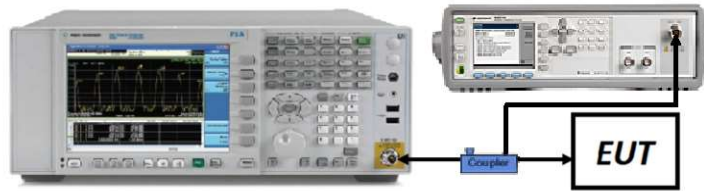
Figure 7-4. Test Instrument & Measurement Setup
