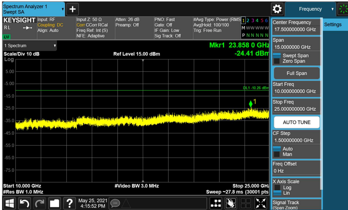
Plot 7-39. Conducted Spurious Plot (Bluetooth, 3Mbps – Ch. 39)
