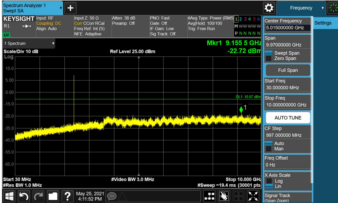
Plot 7-36. Conducted Spurious Plot (Bluetooth, 3Mbps – Ch. 0)
