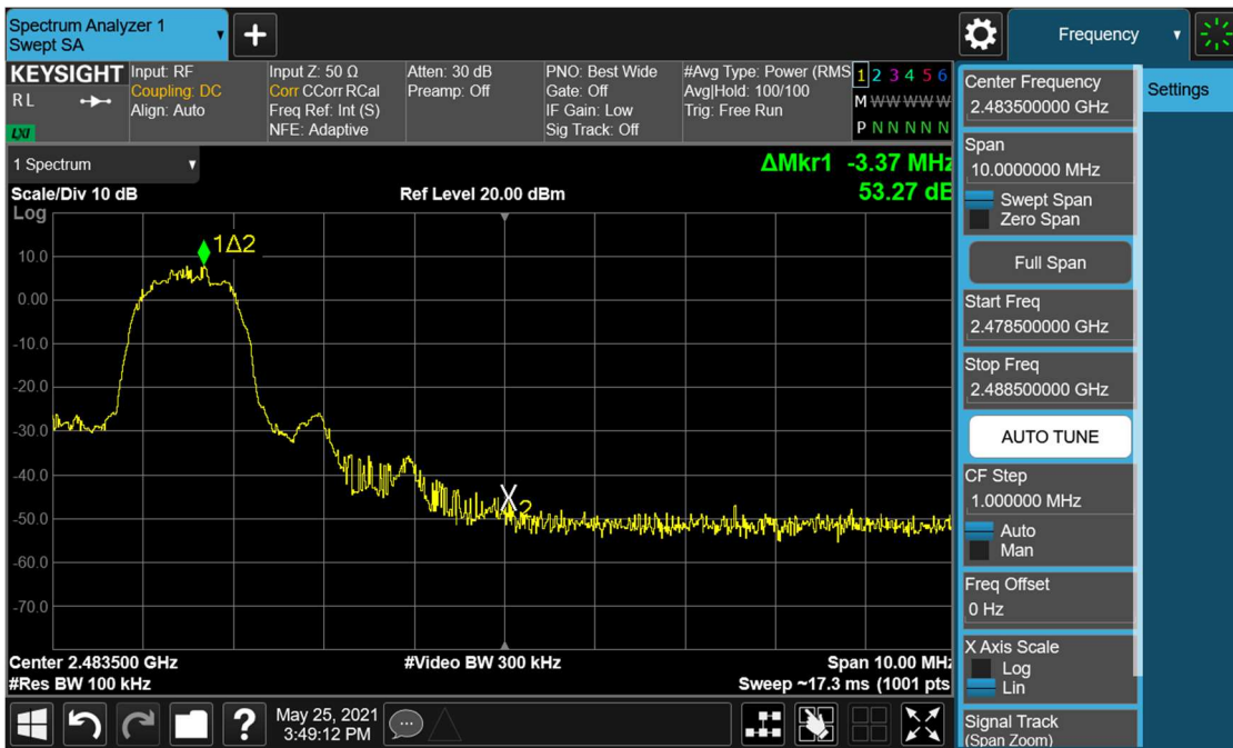
Plot 7-29. Band Edge Plot (Bluetooth with Hopping Disabled, 3 Mbps – Ch. 78)
