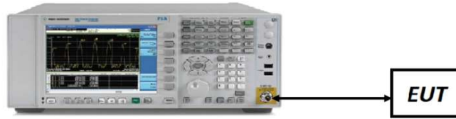
Figure 7-2. Test Instrument & Measurement Setup for Power Measurements
