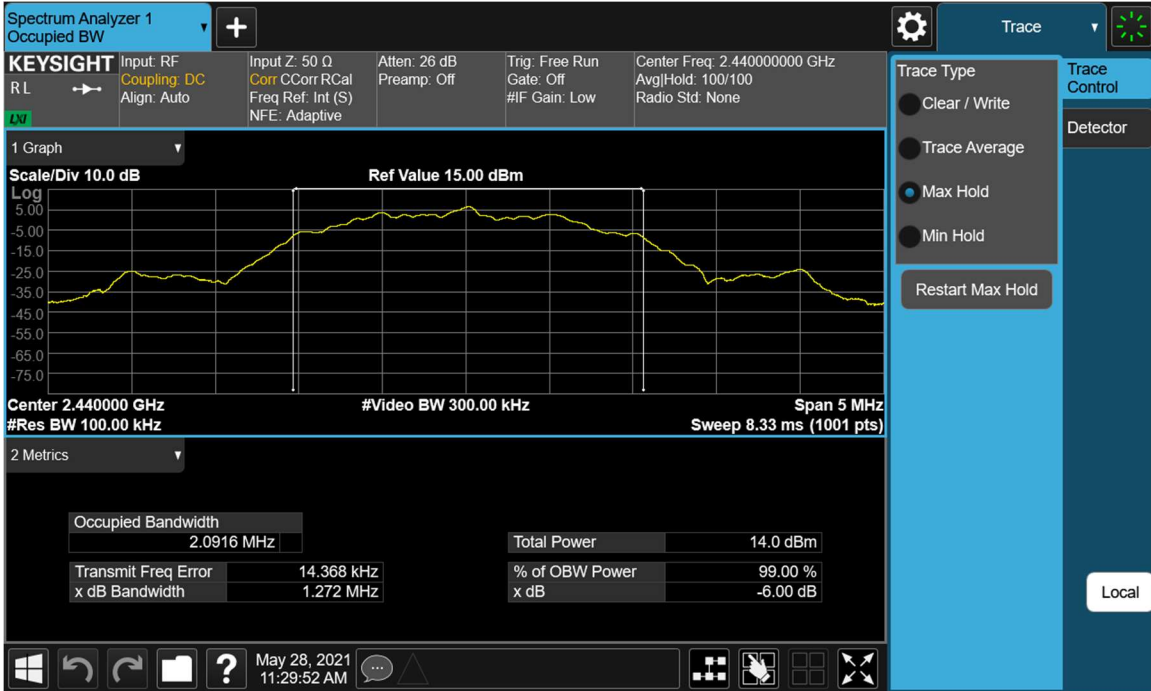
Plot 7-11. 6dB Bandwidth Plot (Bluetooth (LE), 2Mbps – Ch. 19)
