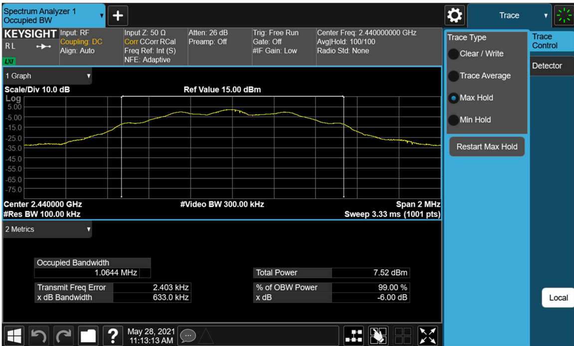
Plot 7-2. 6dB Bandwidth Plot (Bluetooth (LE), 125kbps – Ch. 19)
