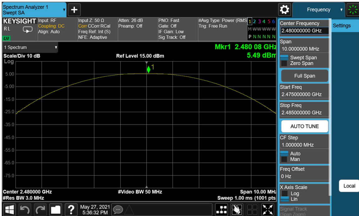
Plot 7-18. Peak Power Plot (Bluetooth (LE), 500kbps – Ch. 39)
