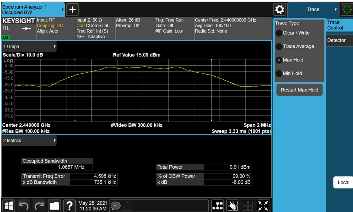
Plot 7-8. 6dB Bandwidth Plot (Bluetooth (LE), 1Mbps – Ch. 19)
