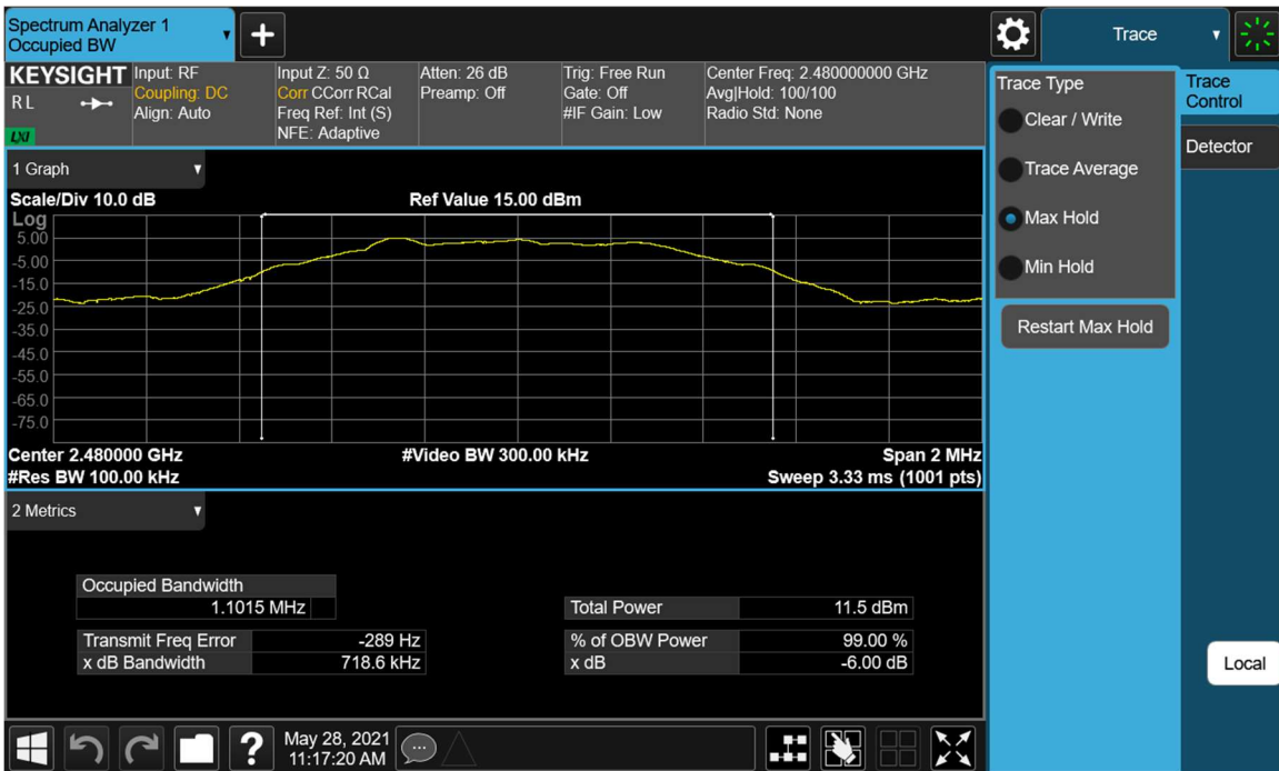
Plot 7-6. 6dB Bandwidth Plot (Bluetooth (LE), 500kbps – Ch. 39)
