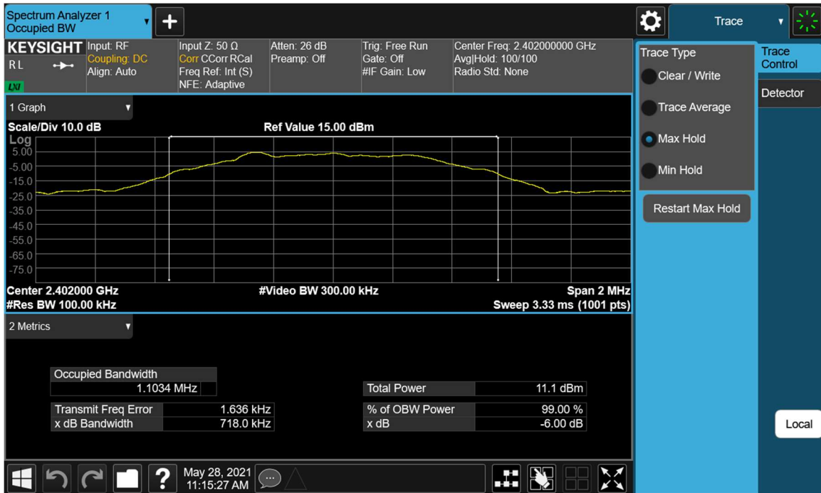
Plot 7-4. 6dB Bandwidth Plot (Bluetooth (LE), 500kbps – Ch. 0)
