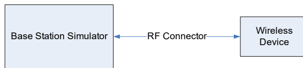
Figure 9-2 Power Measurement Setup
