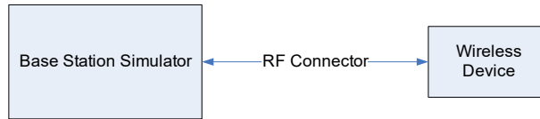
Figure 9-1 Power Measurement Setup
