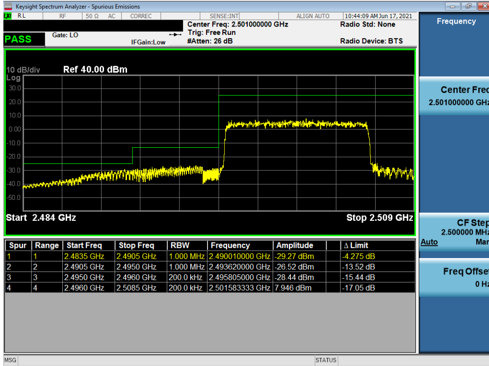
Plot 7-22. Lower ACP Plot (LTE Band 41(PC3) - 10MHz QPSK – Full RB)
