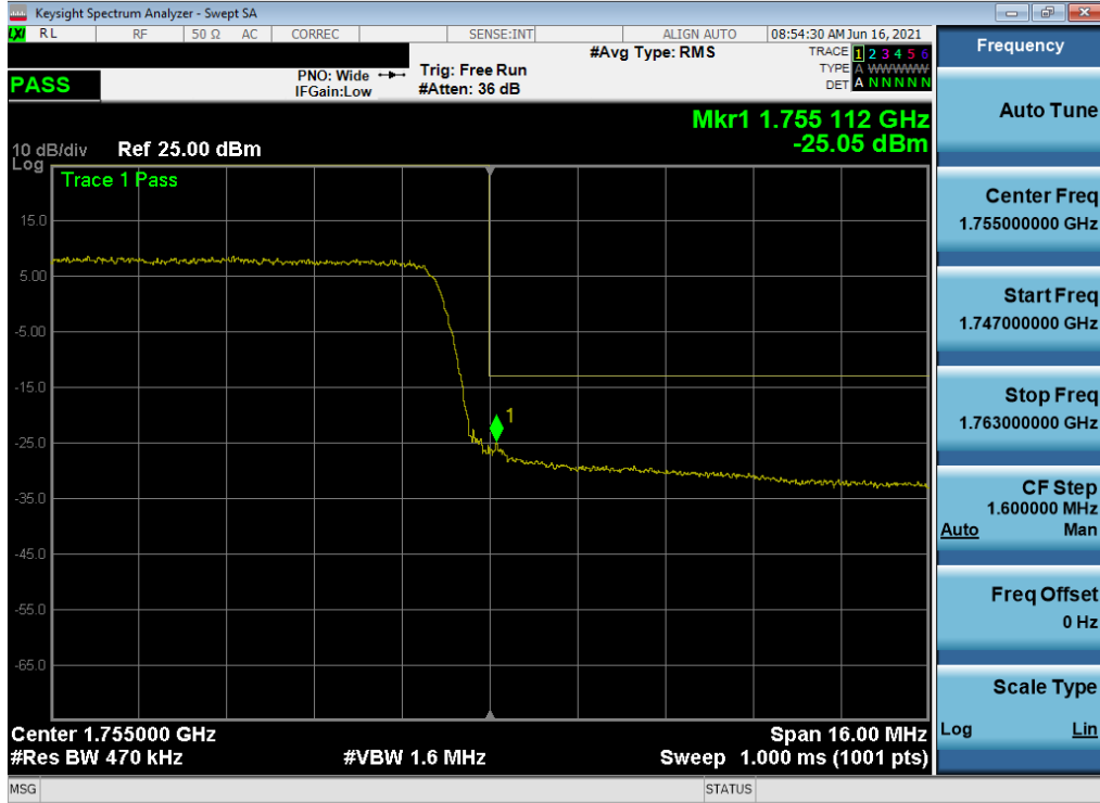
Plot 7-65. Upper Band Edge Plot (LTE Band 4 - 20MHz QPSK – Full RB)
