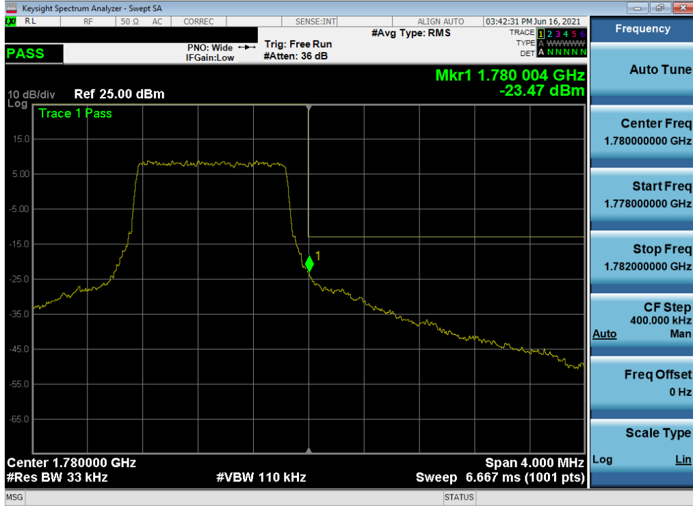
Plot 7-97. Upper Band Edge Plot (LTE Band 66 – 1.4MHz QPSK – Full RB)
