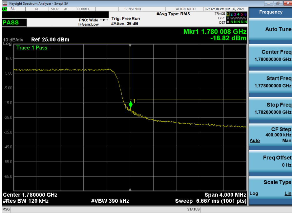
Plot 7-85. Upper Band Edge Plot (LTE Band 66 - 5MHz QPSK – Full RB)
