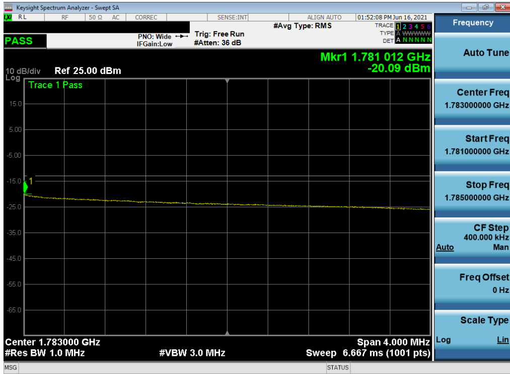
Plot 7-80. Upper Extended Band Edge Plot (LTE Band 66 - 10MHz QPSK – Full RB)
