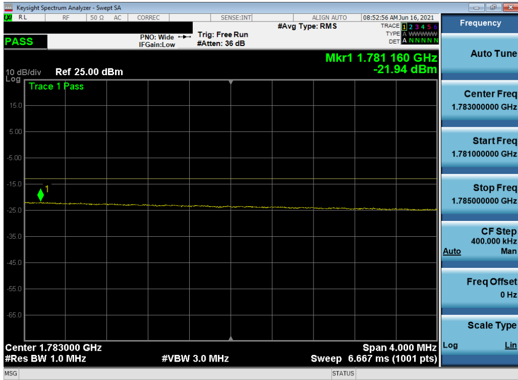
Plot 7-68. Channel Edge Plot (LTE Band 66 - 20MHz QPSK – Full RB)
