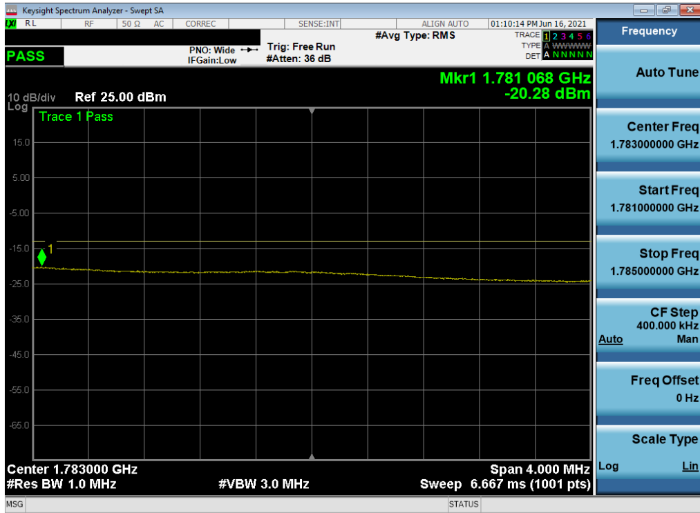
Plot 7-74. Upper Extended Band Edge Plot (LTE Band 66 - 15MHz QPSK – Full RB)
