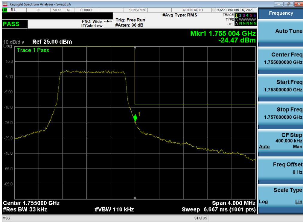
Plot 7-95. Upper Band Edge Plot (LTE Band 4 – 1.4MHz QPSK – Full RB)
