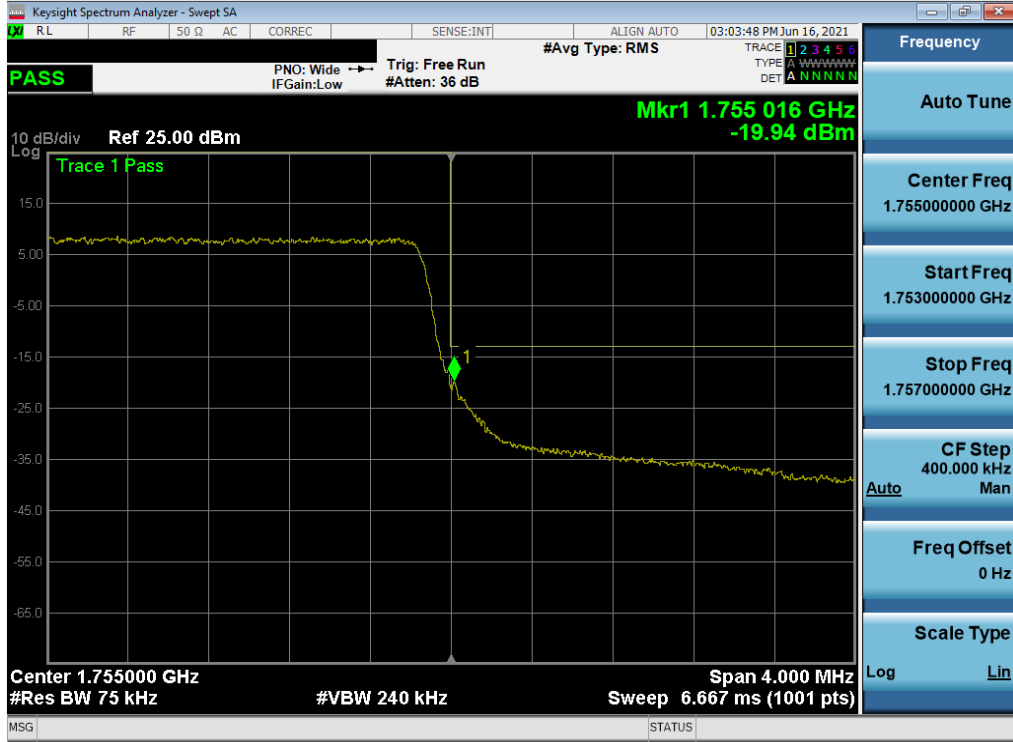
Plot 7-89. Upper Band Edge Plot (LTE Band 4 - 3MHz QPSK – Full RB)
