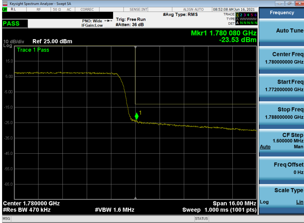
Plot 7-67. Upper Band Edge Plot (LTE Band 66 - 20MHz QPSK – Full RB)
