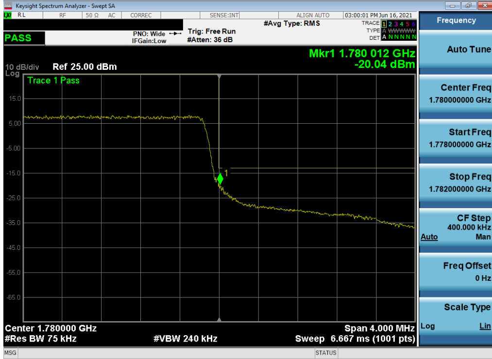
Plot 7-91. Upper Band Edge Plot (LTE Band 66 - 3MHz QPSK – Full RB)
