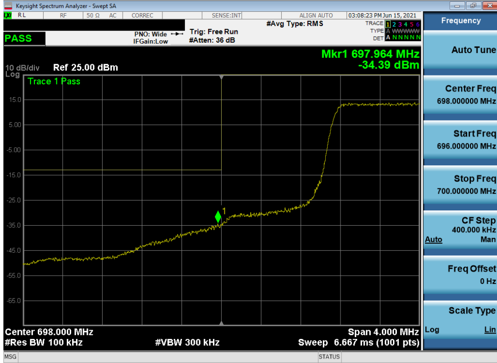
Plot 7-57. Lower Band Edge Plot (LTE Band 12 – 1.4MHz QPSK – Full RB)
