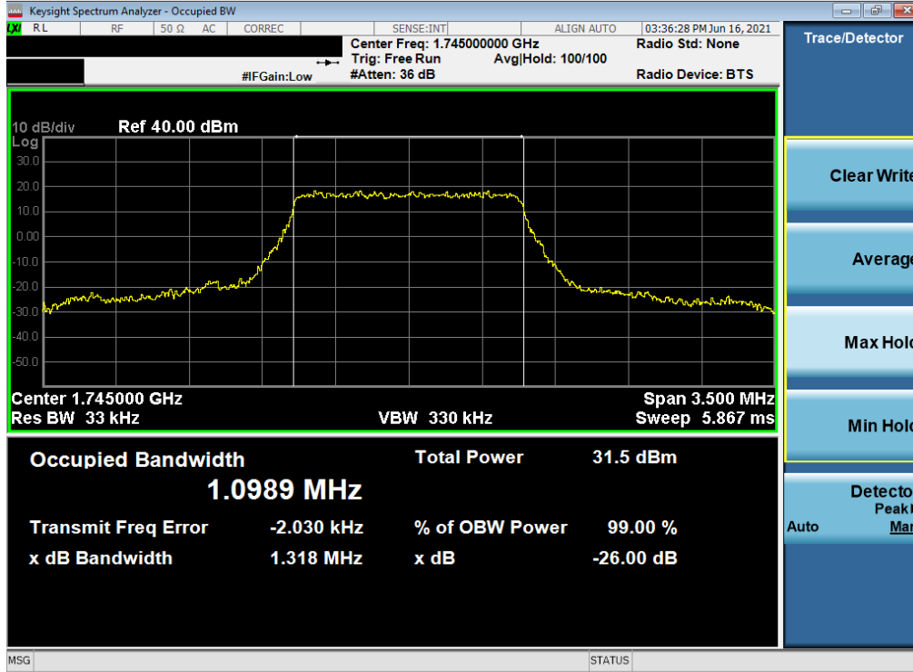
Plot 7-20. Occupied Bandwidth Plot (LTE Band 66/4 - 1.4MHz QPSK - Full RB)
