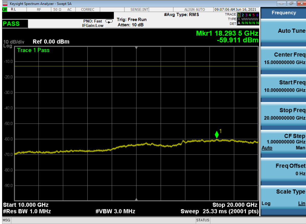
Plot 7-42. Conducted Spurious Plot (LTE Band 66/4 - 20MHz QPSK - 1 RB - Low Channel)
