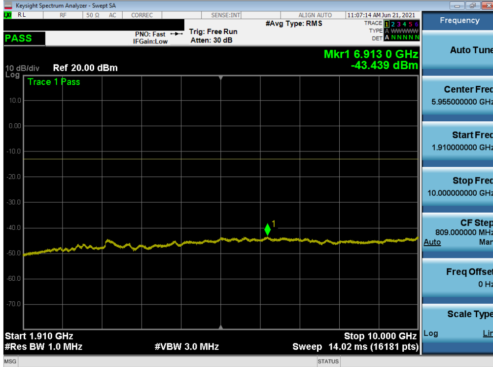
Plot 7-38. Conducted Spurious Plot (WCDMA Ch. 9400)
