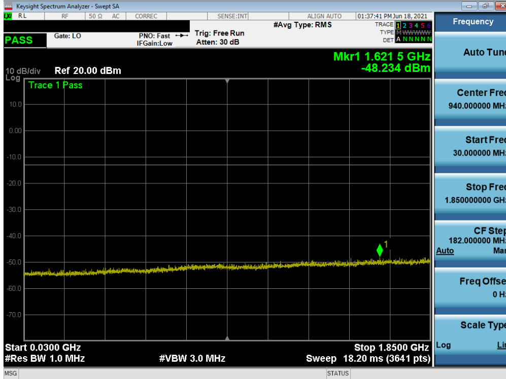
Plot 7-31. Conducted Spurious Plot (GPRS Ch. 810)
