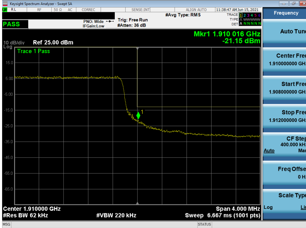
Plot 7-57. Upper Band Edge Plot (LTE Band 2 - 5MHz QPSK – Full RB)
