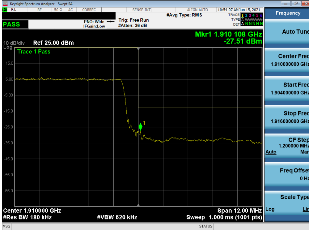
Plot 7-49. Upper Band Edge Plot (LTE Band 2 - 15MHz QPSK – Full RB)
