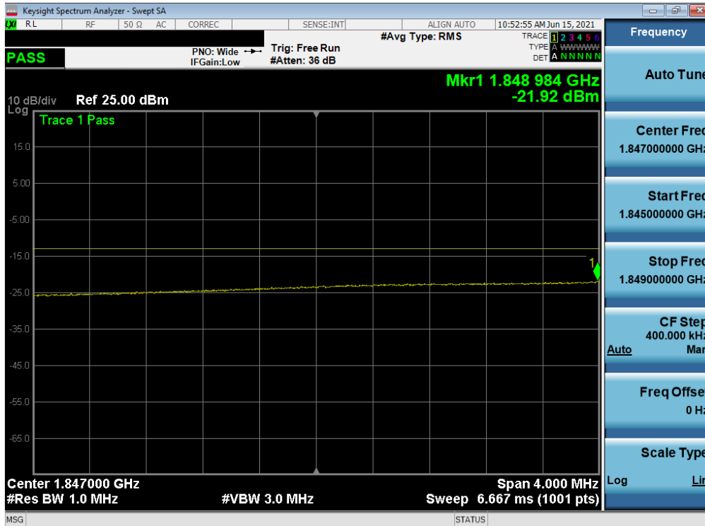
Plot 7-48. Extended Lower Band Edge Plot (LTE Band 2 - 15MHz QPSK – Full RB)
