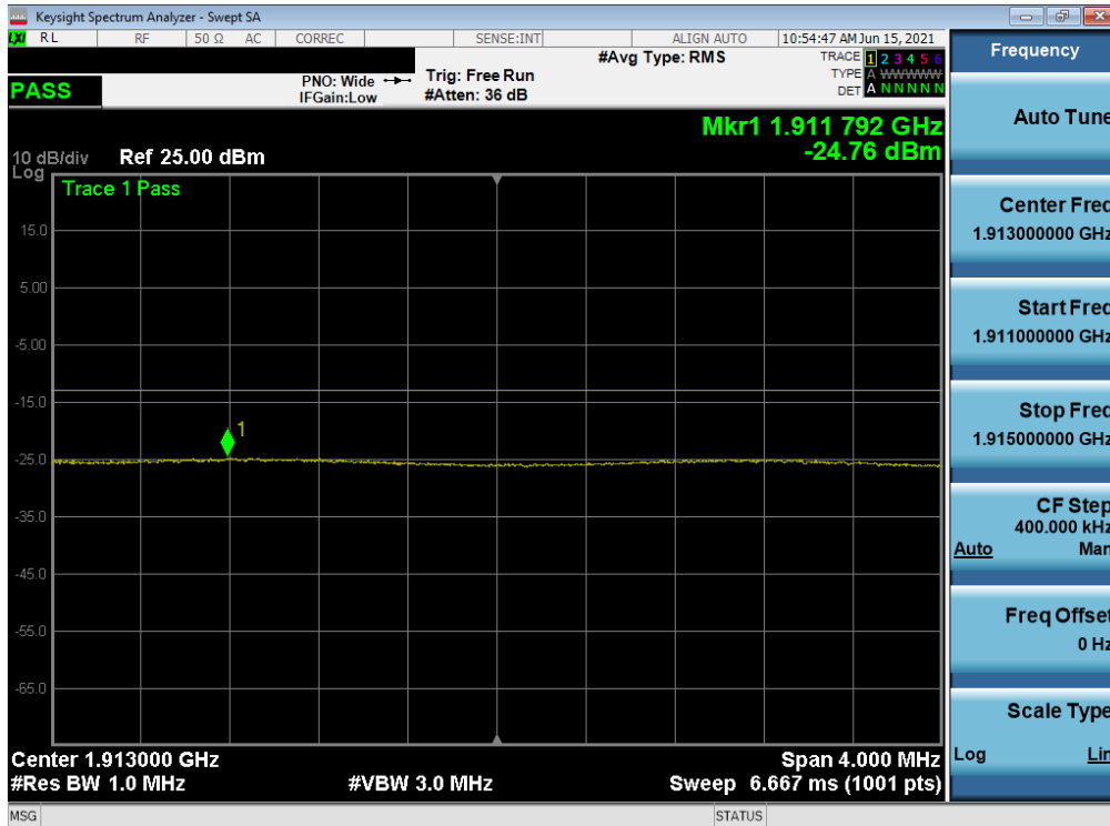
Plot 7-50. Extended Upper Band Edge Plot (LTE Band 2 - 15MHz QPSK – Full RB)
