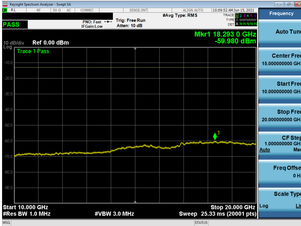
Plot 7-18. Conducted Spurious Plot (LTE Band 2 - 20MHz QPSK - 1RB - Low Channel)
