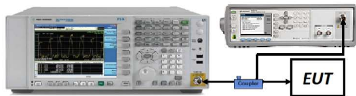
Figure 7-7. Test Instrument & Measurement Setup
