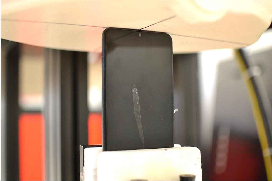
SAR Test Setup Photo 13 – Phablet, Top Edge at 0 mm
