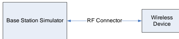
Figure 9-1 Power Measurement Setup
