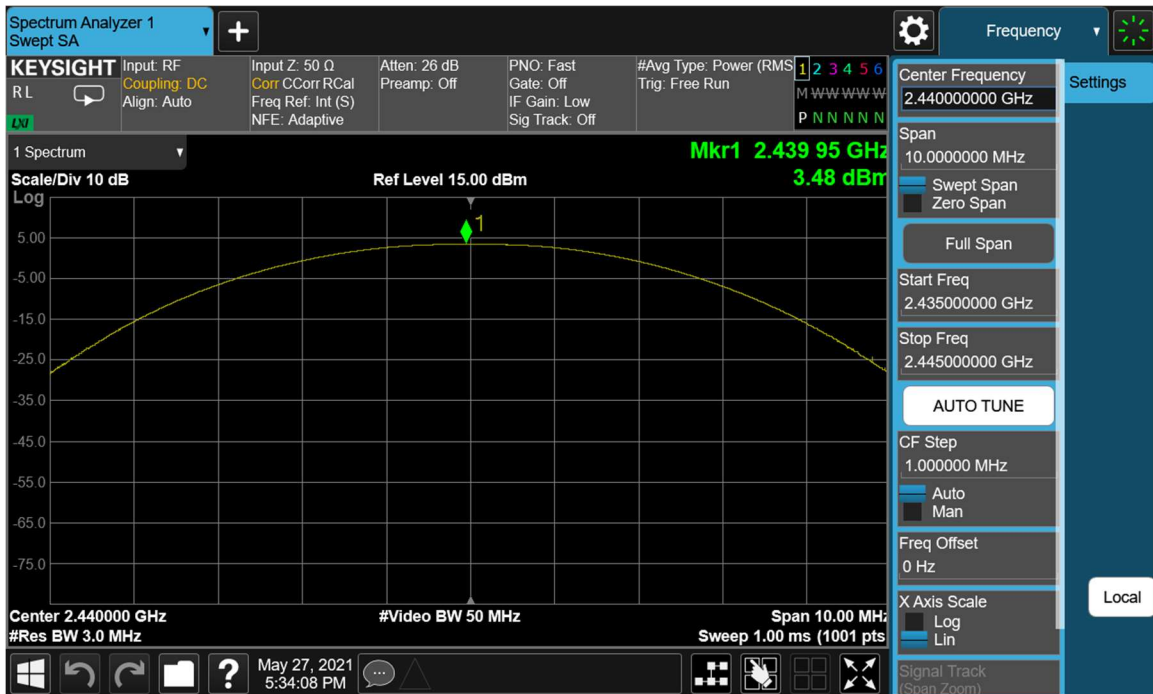
Plot 7-14. Peak Power Plot (Bluetooth (LE), 125kbps – Ch. 19)
