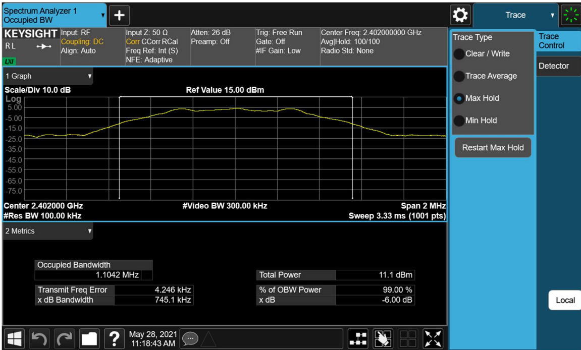
Plot 7-7. 6dB Bandwidth Plot (Bluetooth (LE), 1Mbps – Ch. 0)
