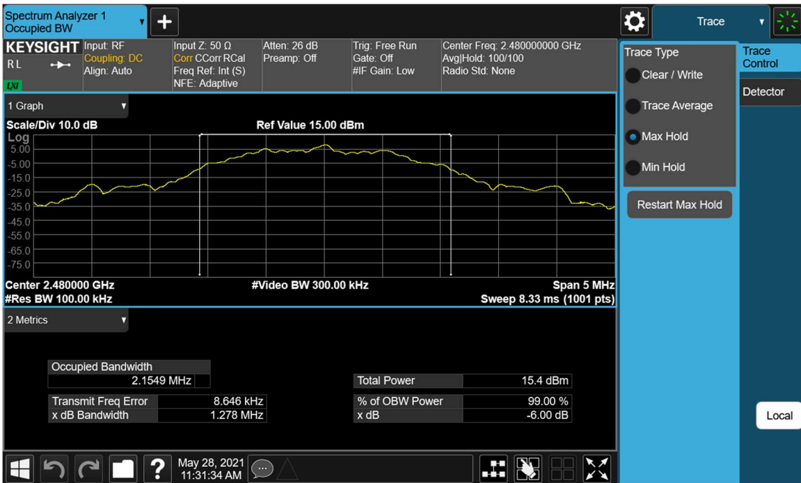
Plot 7-12. 6dB Bandwidth Plot (Bluetooth (LE), 2Mbps – Ch. 39)
