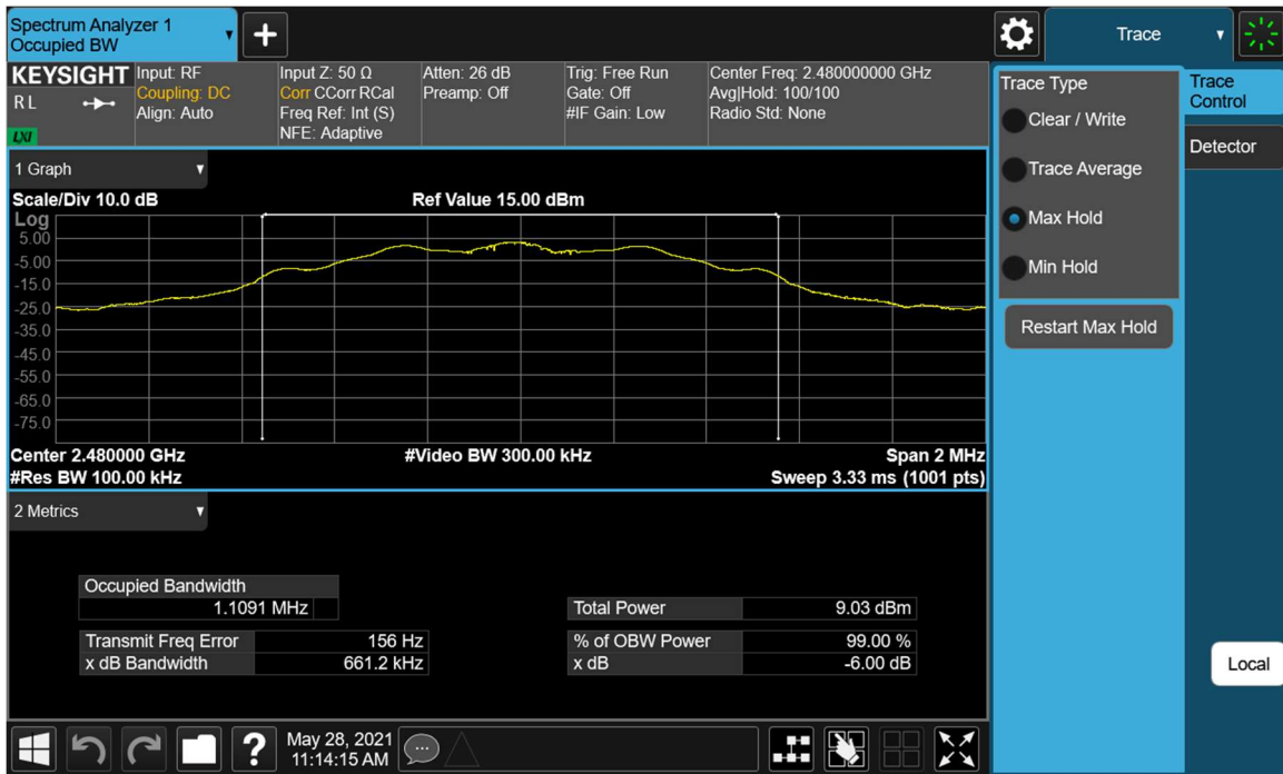
Plot 7-3. 6dB Bandwidth Plot (Bluetooth (LE), 125kbps – Ch. 39)
