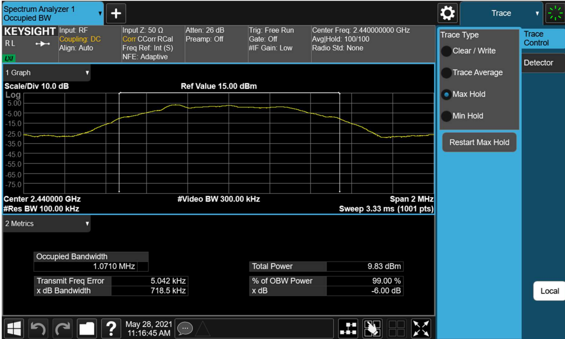
Plot 7-5. 6dB Bandwidth Plot (Bluetooth (LE), 500kbps – Ch. 19)
