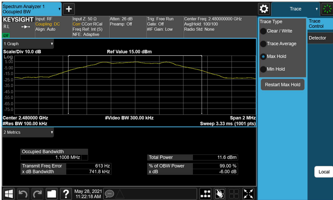
Plot 7-9. 6dB Bandwidth Plot (Bluetooth (LE), 1Mbps – Ch. 39)
