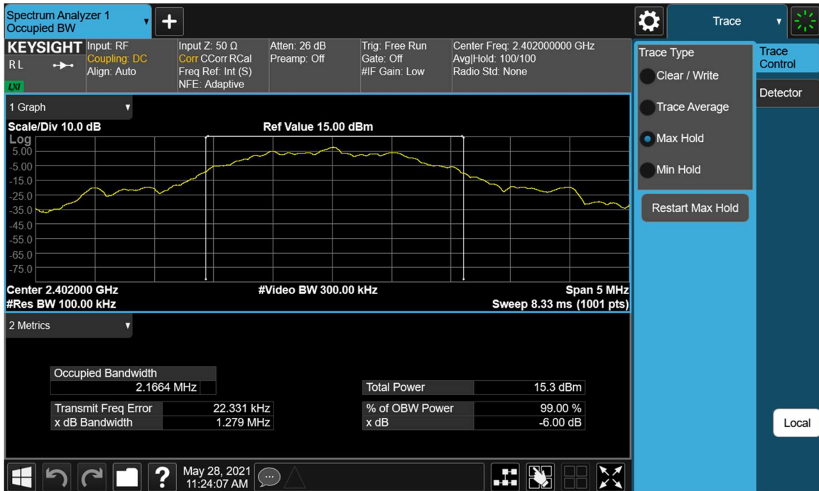
Plot 7-10. 6dB Bandwidth Plot (Bluetooth (LE), 2Mbps – Ch. 0)
