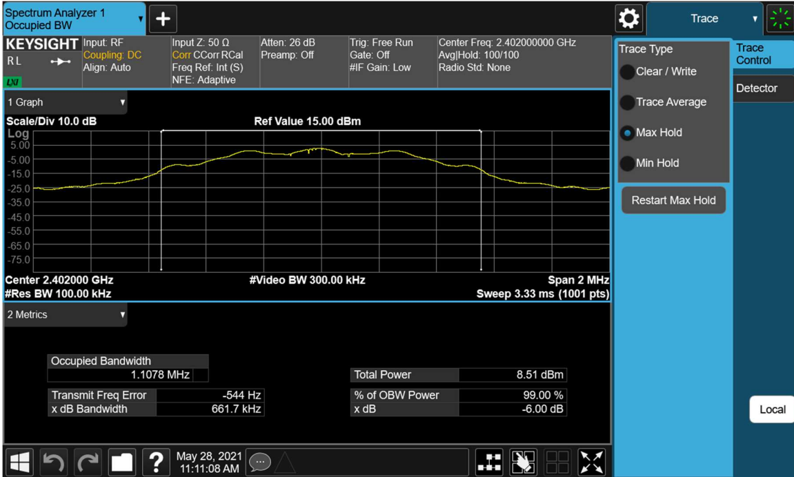
Plot 7-1. 6dB Bandwidth Plot (Bluetooth (LE), 125kbps – Ch. 0)
