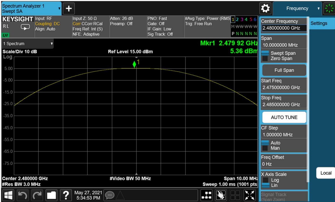
Plot 7-15. Peak Power Plot (Bluetooth (LE), 125kbps – Ch. 39)
