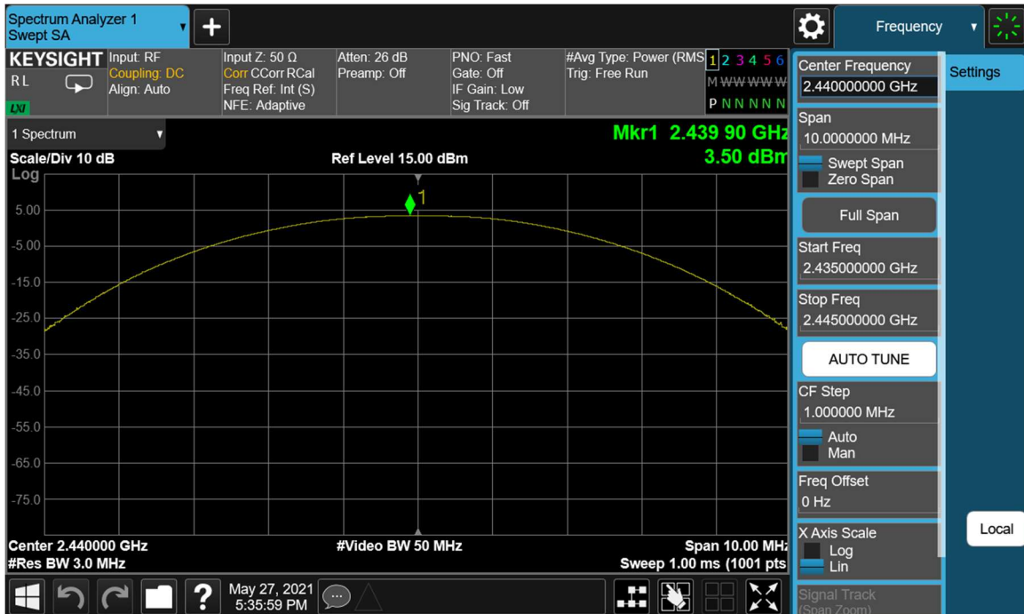
Plot 7-17. Peak Power Plot (Bluetooth (LE), 500kbps – Ch. 19)
