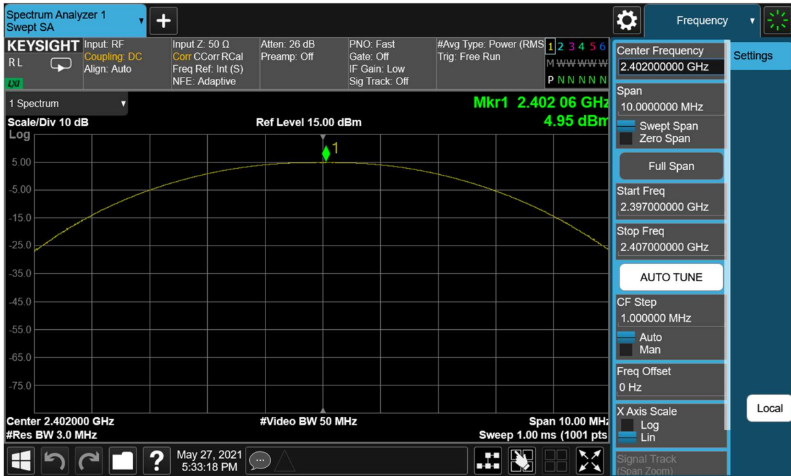
Plot 7-13. Peak Power Plot (Bluetooth (LE), 125kbps – Ch. 0)
