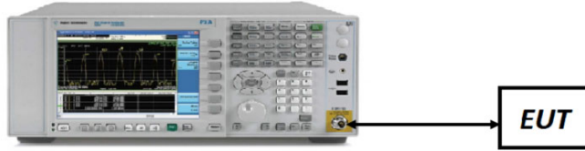
Figure 7-2. Test Instrument & Measurement Setup for Power Measurements
