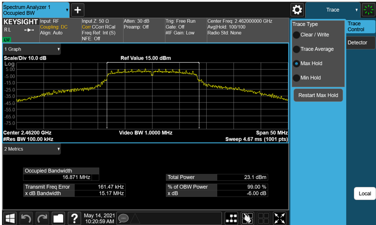
Plot 7-6. 6dB Bandwidth Plot SISO ANT1 (802.11g – Ch. 11)
