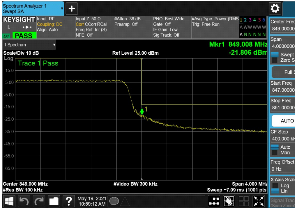
Plot 7-42. Upper Band Edge Plot (LTE Band 5 - 5MHz QPSK – Full RB)
