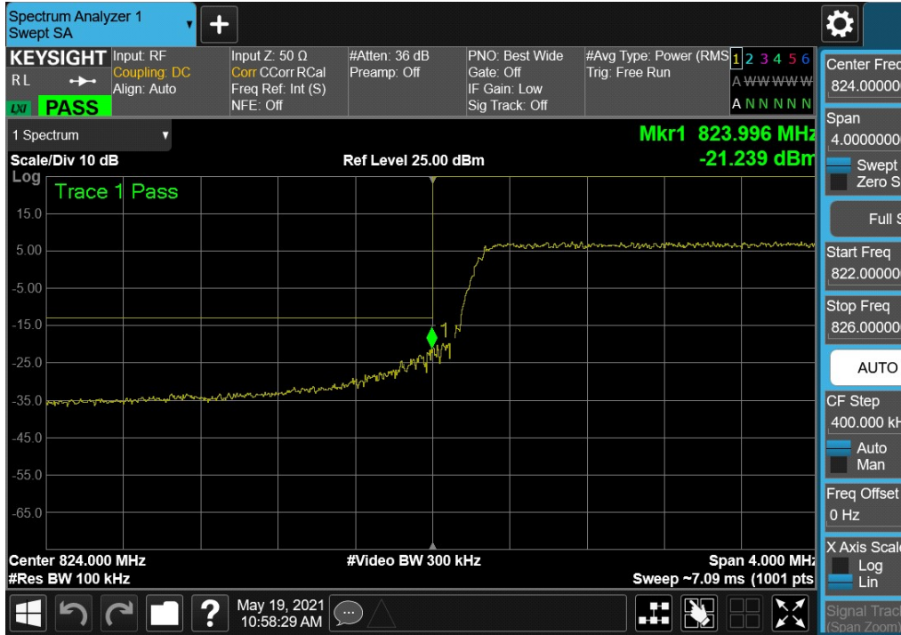
Plot 7-41. Lower Band Edge Plot (LTE Band 5 - 5MHz QPSK – Full RB)
