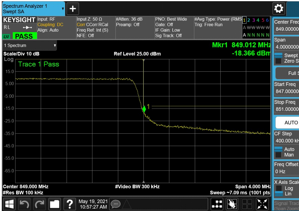
Plot 7-44. Upper Band Edge Plot (LTE Band 5 - 3MHz QPSK – Full RB)
