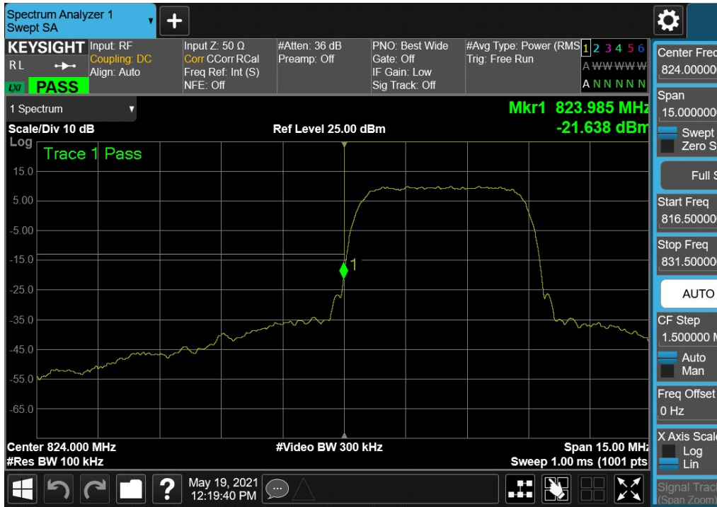
Plot 7-49. Lower Band Edge Plot (WCDMA Cell – Ch. 4132)
