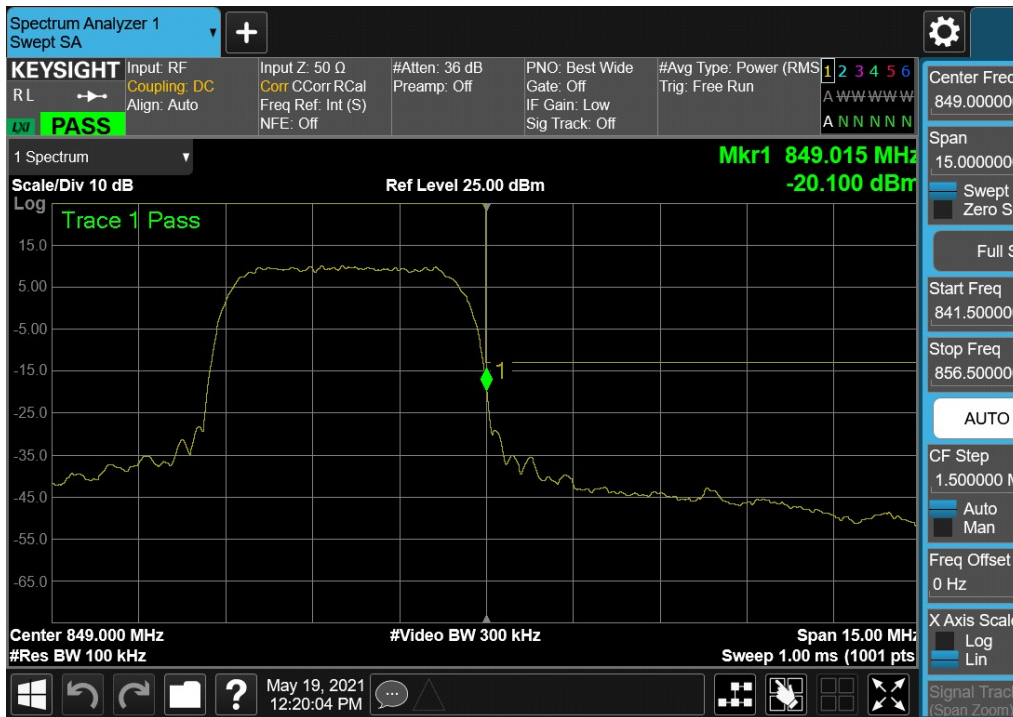
Plot 7-50. Upper Band Edge Plot (WCDMA Cell – Ch. 4233)
