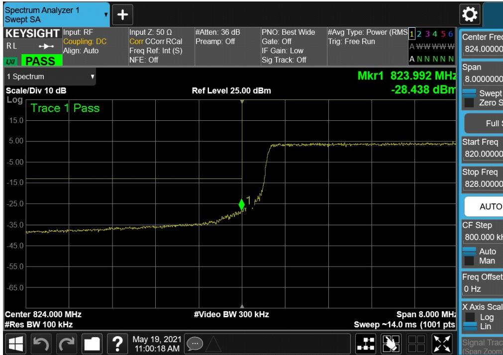
Plot 7-39. Lower Band Edge Plot (LTE Band 5 - 10MHz QPSK – Full RB)
