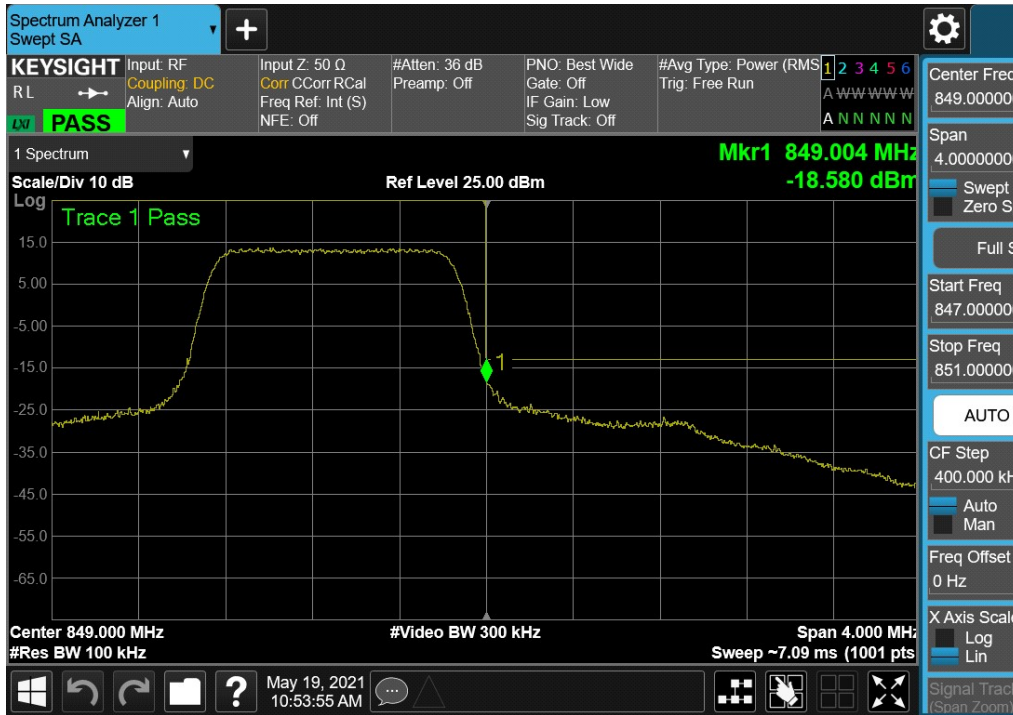
Plot 7-46. Upper Band Edge Plot (LTE Band 5 – 1.4MHz QPSK – Full RB)
