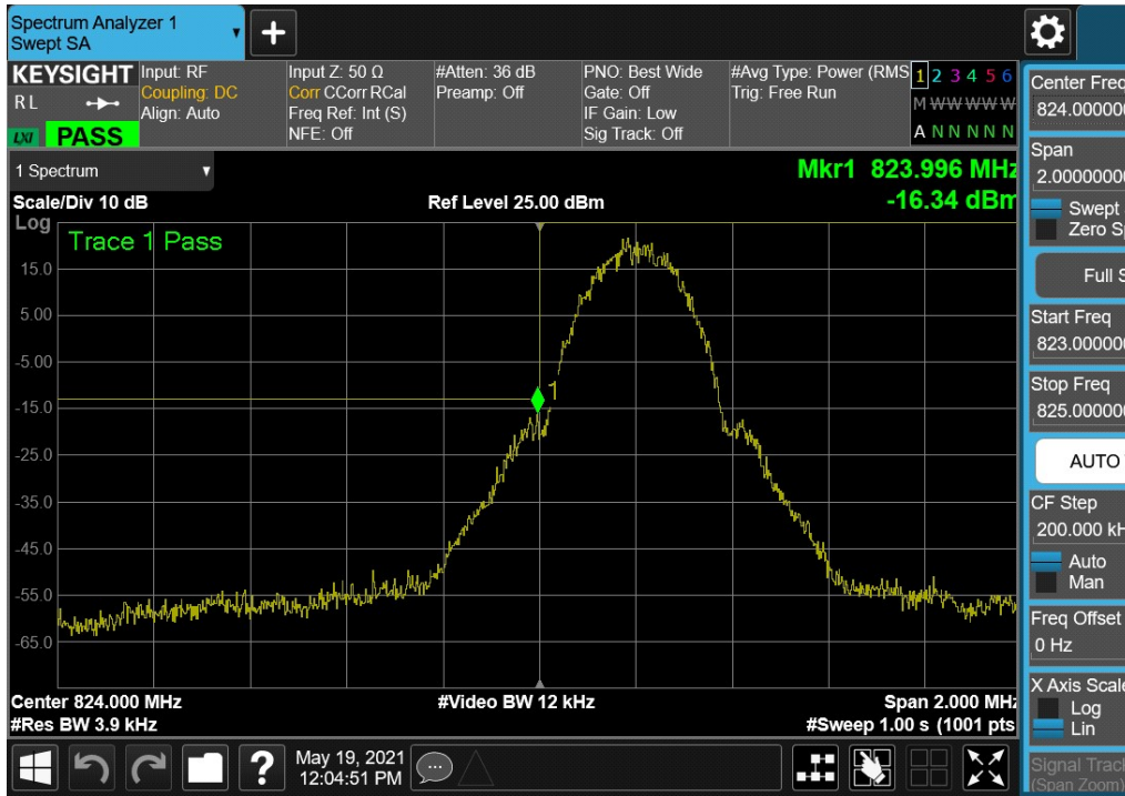
Plot 7-47. Lower Band Edge Plot (GPRS Cell – Ch. 128)
