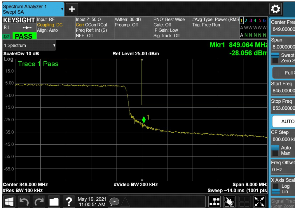
Plot 7-40. Upper Band Edge Plot (LTE Band 5 - 10MHz QPSK – Full RB)
