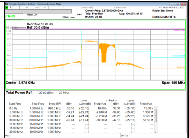
LTE B41 15MHz + 15MHz 16QAM High Ch RB75-0 + RB75-0
