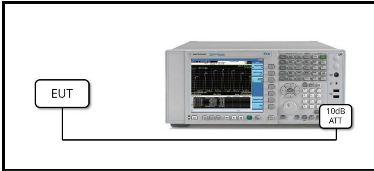
**SETUP DIAGRAM FOR TESTS (RADIATED TEST SETUP)**
