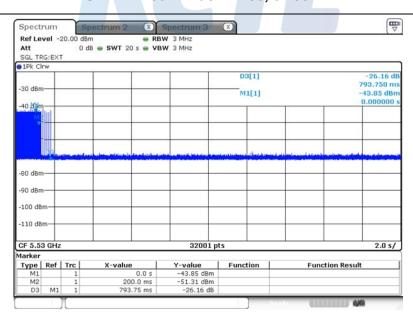
Channel move time = 0.79375 sClosing time =  $0.000625 \text{ s} \times 85 = 0.053125 \text{ s}$
