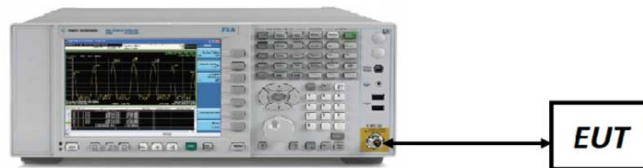
Figure 7-5. Test Instrument & Measurement Setup
