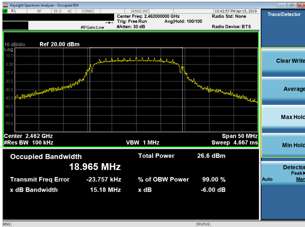
Plot 7-9. 6dB Bandwidth Plot (802.11n (2.4GHz) – Ch. 11)
