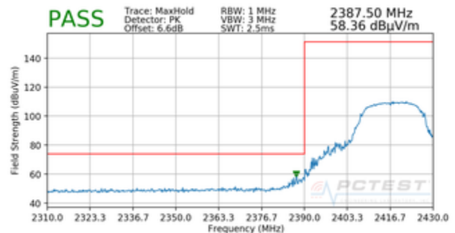
Plot 7-44. Radiated Restricted Lower Band Edge Measurement (Peak)
