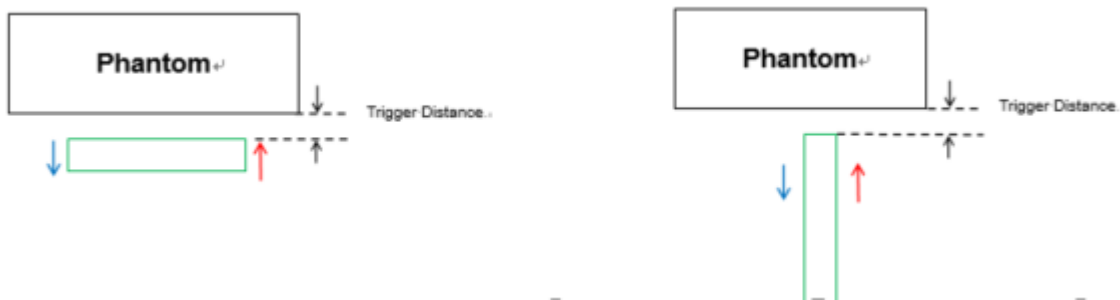
Proximity Sensor Trigger Distance Assessment KDB 616217 D04§6.2
