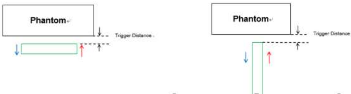
Proximity Sensor Trigger Distance Assessment KDB 616217 D04§6.2
