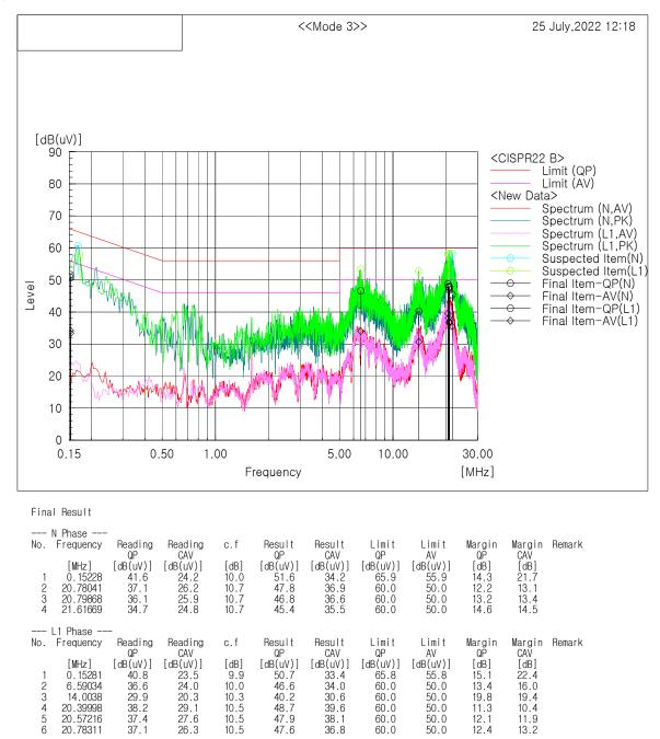
Note 1) Two graphs measured for both Live(L1) and Neutral(N) of the LISN are combined into one graph Note 2) Level (QP and/or CAV) = Meter Reading (QP and/or CAV) + Corr. (LISN Insertion Loss + Cable Loss) Margin (QP and/or CAV) = Limit – Level (QP and/or CAV)
