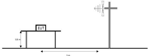
The diagram below shows the test setup that is utilized to make the measurements for emission from 1  $\oplus$  to the tenth harmonic of the highest fundamental frequency or to 40  $\oplus$  emissions, whichever is lower.
