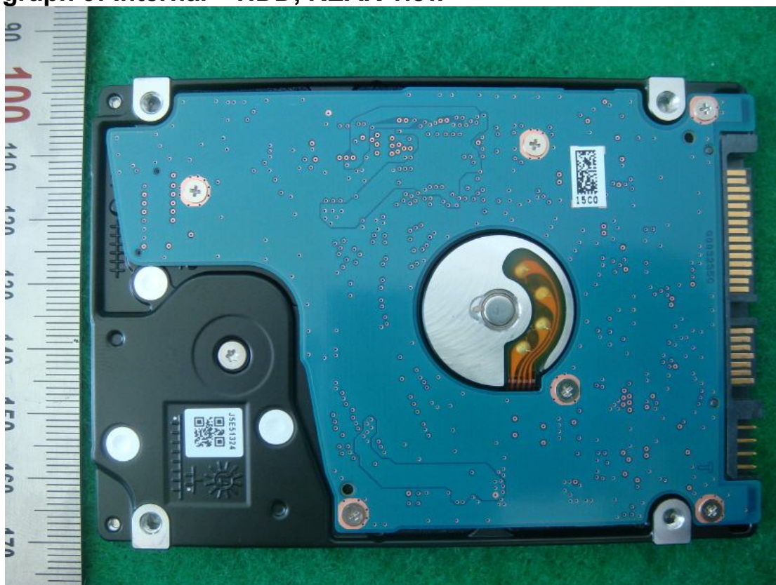
Photograph 9: Internal – HDD, REAR view
