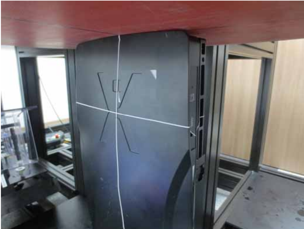
Top from Flat Phantom (Separation Distance: 0 cm)
