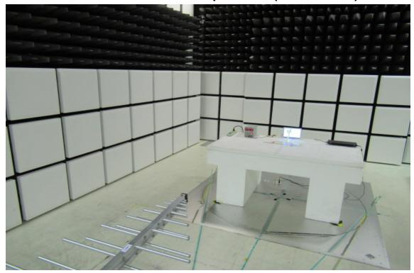
Radiated Emission Set up Photos (Above 1GHz)
